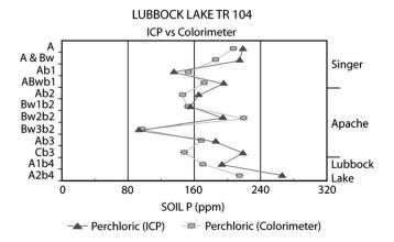
Fig. 6. Comparison of perchloric acid extractions from Lubbock Lake, Trench 104 samples measured by ICP vs. colorimetry.
