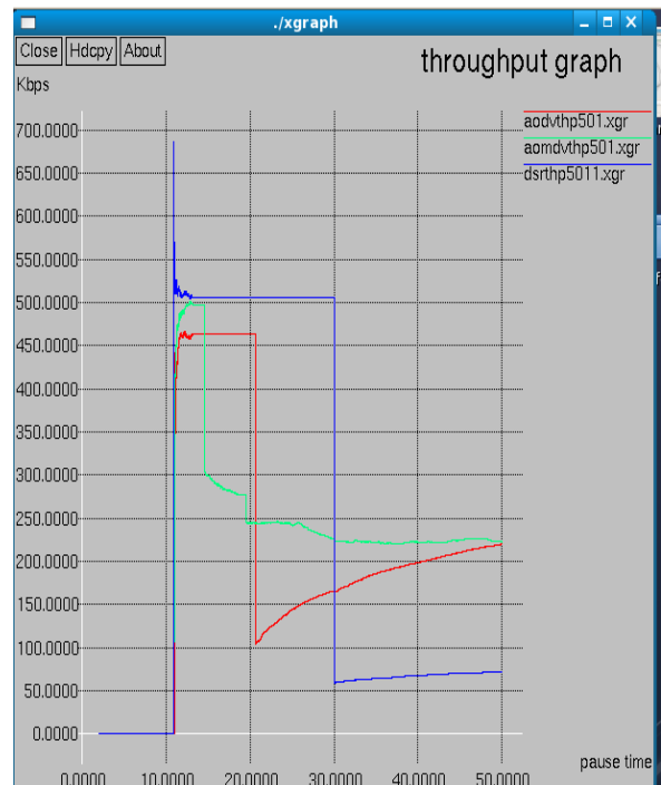
5.3 Comparison of AODV, AOMDV and DSR on basis of Throughput at maximum connection 50
