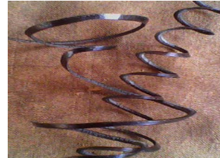
Plate 1. Micrograph of steel chips at 250 rpm, 1 mm depth of cut
