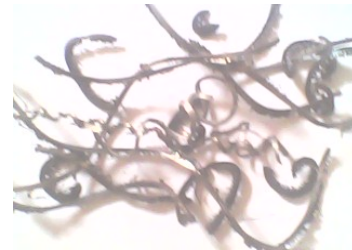
Plate 11. Micrograph of steel chips 25% soluble oil
