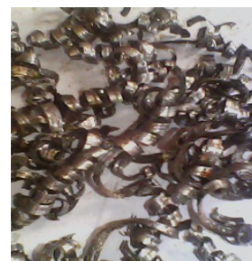
Plate 4. Micrograph of steel chips at 100 % Water Melon oil
