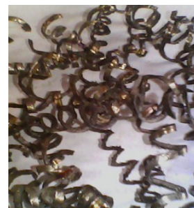
Plate 3. Micrograph of steel chips at 100 % Neem oil
