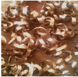
Plate 6. Micrograph of steel chips at 50 % Neem oil
