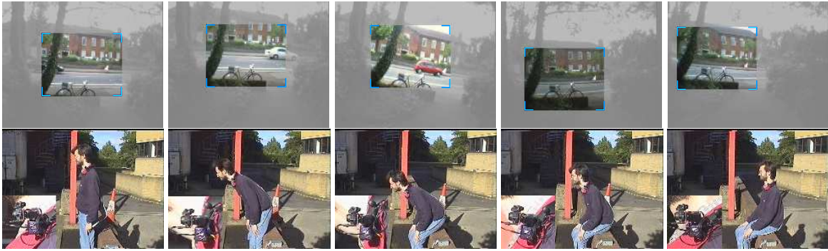
Figure 5: Comparable samples from sequences obtained while the user sits down in an outdoor scene (bottom row). The top row shows the view and fovea when the camera is passive, the second row when it is active and the third row for the configuration with active plus software-controlled fovea. Note that the passive camera loses the initial target point for about half the sequence.
