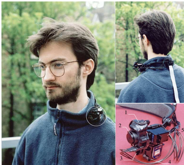
Figure 1: 3-axis Wearable Visual Robot. Closeup: 1) 2D Accelerometer. 2) CMOS Color Camera. 3) Elevation axis. 4) Pan axis. 5) Cyclotorsion axis.
