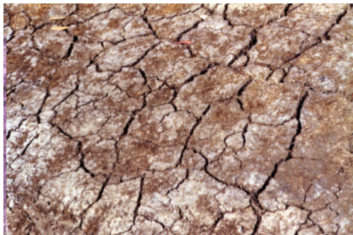
Figure 1.6 Fracture in clay matrix due to wetting and drying cycles.
