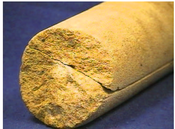
Figure 2.11 Close-up of fracture in sandstone core
