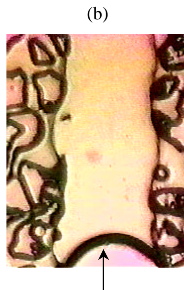
Figure 6.1 Observation of three-phase flow in a fracture, simulated with a micromodel.
