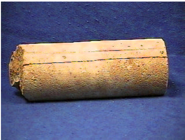
Figure 2.10 Image of fractured sandstone core
