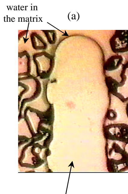
Figure 6.1 Observation of three-phase flow in a fracture, simulated with a micromodel.
