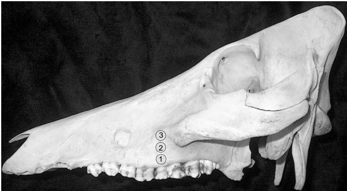
Figure 4-1. Diagram of gage placement. 1) Inferior alveolar rosette, 2) Intermediate alveolar rosette, 3) Facial rosette.
