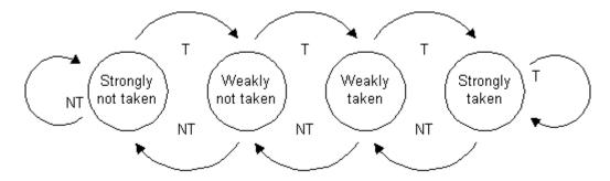
Figure 3.1. Saturating 2-bit counter
