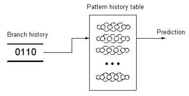
Figure 3.2. Adaptive two-level predictor
