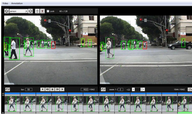
Fig. 3. The annotation tool allows annotators to efficiently navigate and annotate a video in a minimum amount of time. Its most salient aspect is an interactive procedure where the annotator labels only a sparse set of frames and the system automatically predicts pedestrian positions in intermediate frames. The annotation tool is available on the project website.
