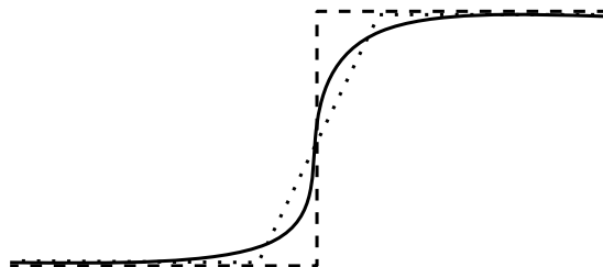
Figure 14.3: Step-like McCulloch-Pitts input/output function ( dashed ), a high-gain sigmoid function ( solid ), and a piecewise linear function ( dotted ).
