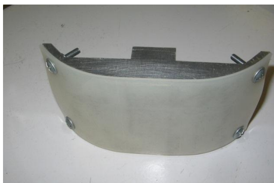
Test foot with clamping screws
