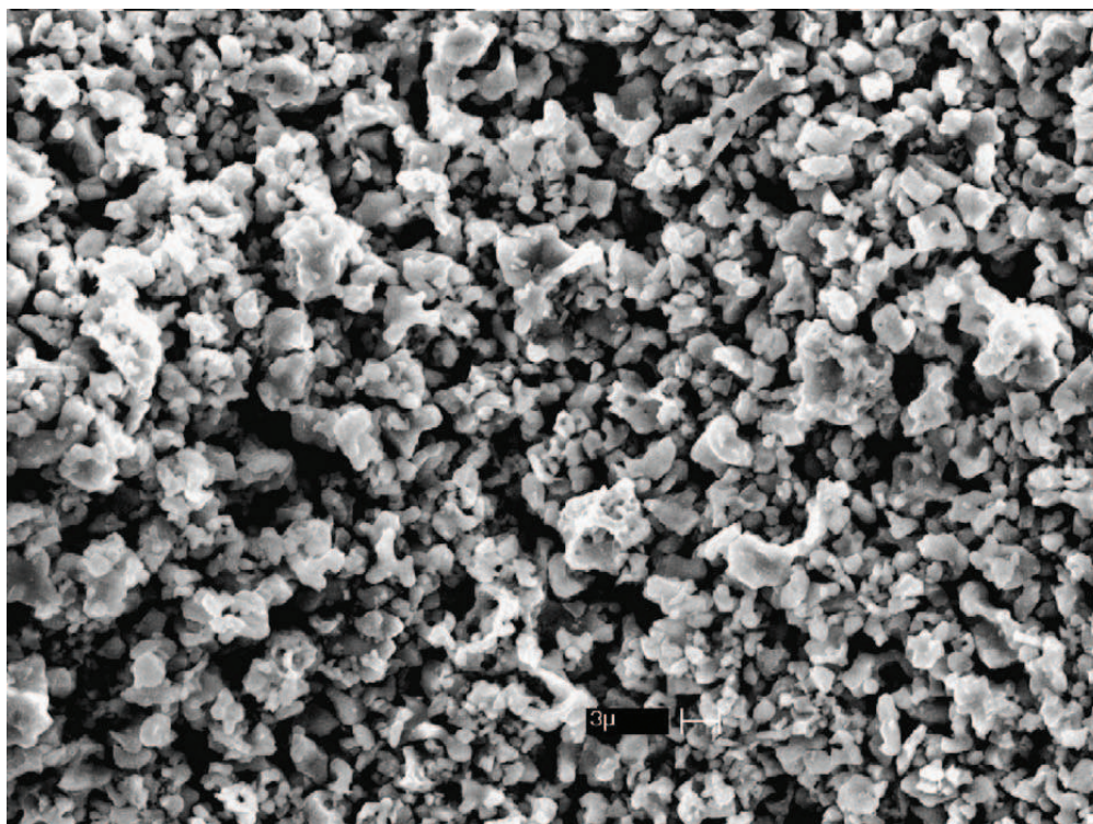
SEM photo of LiFePO 4 powders ( G.X. Wang et al. / Electrochimica Acta 50 (2004) 443–447 )
