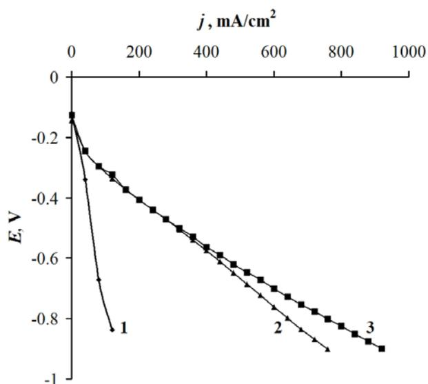
**Figure 4.** Dependence of potential on current density for oxygen electrodes with the active layer in an amount of  $0.02 \text{ g/cm}^2$  consisting of initial MWCNTs (1) and RGO which were reduced by the sodium hypophosphite from MWCNTs oxidized with potassium dichromate (2) and potassium permanganate (3)
