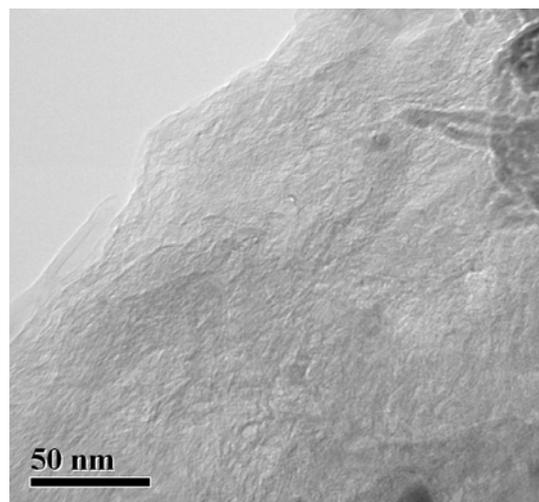
**Figure 1.** Micrograph of a sample of RGO obtained from MWCNTs oxidized by KMnO<sub>4</sub> and reduced with sodium sulfite
