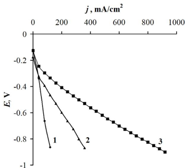
Figure 6. Dependence of potential on current density for oxygen electrodes with the active layer in an amount of  $0.02\text{ g/cm}^2$  consisting of initial MWCNTs (1) and MWCNTs oxidized with potassium permanganate which were reduced to RGO with sodium sulfite (2) and sodium hypophosphite (3)
