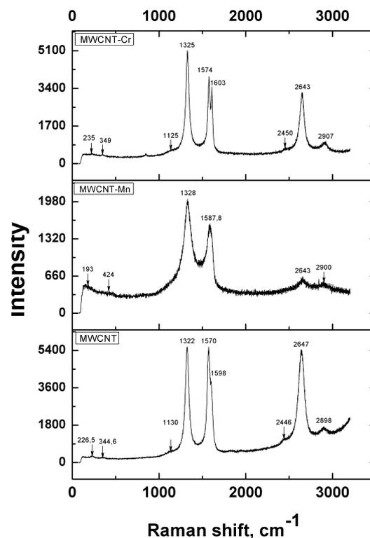
**Figure 5.** Raman spectra obtained at  $633 \text{ nm}$  and the intensity of 50% for initial MWCNTs (MWCNT) and RGO reduced by sodium hypophosphite from the nanotubes oxidized with potassium dichromate (MWCNT – Cr) and potassium permanganate (MWCNT – Mn)
