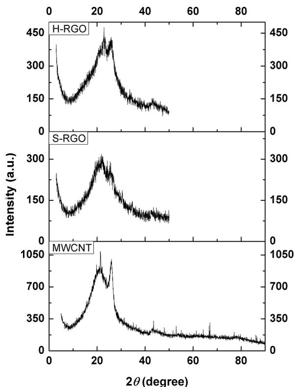
**Figure 3.** X-ray diagram of samples of graphene oxide reduced: (H-RGO) with sodium hypophosphite, (S-RGO) with sodium sulfite, (MWCNT) initial MWCNTs
