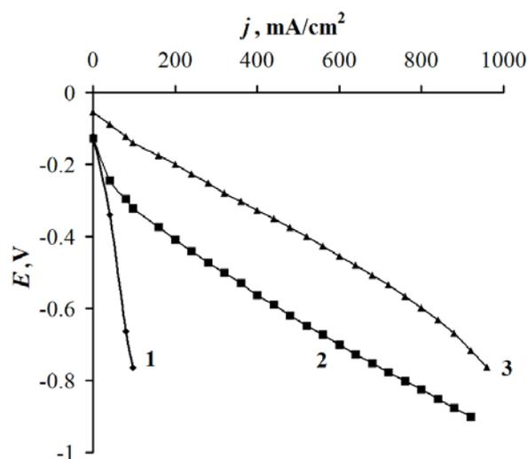
Figure 7. Dependence of potential on current density for oxygen electrodes with the active layer in an amount of  $0.02\text{ g/cm}^2$  consisting of initial MWCNTs (1), RGO obtained by the reduction of sodium hypophosphite MWCNTs oxidized with potassium permanganate (2), MWCNTs with deposited metallic platinum in an amount of 10 wt%
