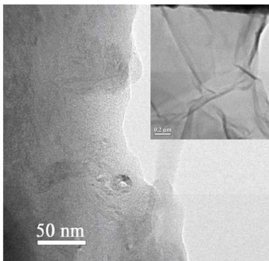
**Figure 2.** Micrograph of a sample of RGO obtained from MWCNTs oxidized by KMnO<sub>4</sub> and reduced with sodium hypophosphite
