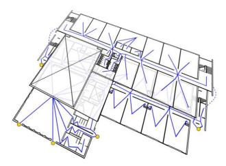
Fig. 2. The representation of a multi-fbor environment used for deployment of the beacons. The yellow dots mark the emergency exits, note the dotted line segments indicate the stairway connections in the planar topological overlay. Assignment considers where the robots are currently positioned ensuring that the distance traveled is minimized wherever possible.
