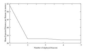
Fig. 7. The mean distance a human will travel (based on the simple fbw model described in the text) as a function of the number of deployed beacons. This is a function of the *locations* of the beacons, too; this plot is for the five locations chosen by the described allocation algorithm.
