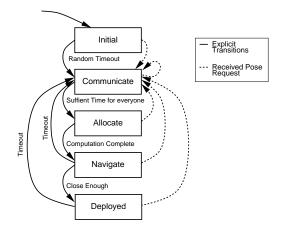
Fig. 4. The Internal State Transition Diagram representation for the robot coordination process. The signal that indicates that a pose request has entered the system is set via another process.
