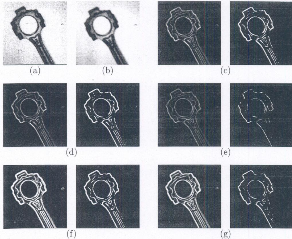
Figure 5.6: A comparison of various edge detectors on a noisy image. (a) Noisy image. (b) Filtered image. (c) Simple gradient using  $1 \times 2$  and  $2 \times 1$  masks,  $T = 32$ . (d) Gradient using  $2 \times 2$  masks,  $T = 64$ . (e) Roberts cross operator,  $T = 64$ . (f) Sobel operator,  $T = 225$ . (g) Prewitt operator,  $T = 225$ .
