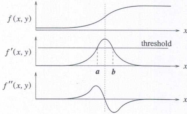
Figure 5.8: If a threshold is used for detection of edges, all points between  $a$  and  $b$  will be marked as edge pixels. However, by removing points that are *not* a local maximum in the first derivative, edges can be detected more accurately. This local maximum in the first derivative corresponds to a zero crossing in the second derivative.
