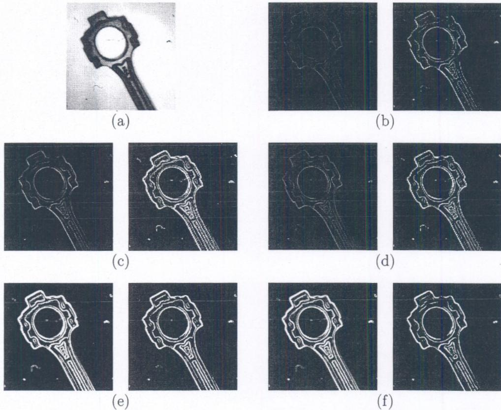
Figure 5.5: A comparison of various edge detectors without filtering. (a) Original image. (b) Simple gradient using  $1 \times 2$  and  $2 \times 1$  masks,  $T = 64$ . (c) Gradient using  $2 \times 2$  masks,  $T = 64$ . (d) Roberts cross operator,  $T = 64$ . (e) Sobel operator,  $T = 225$ . (f) Prewitt operator,  $T = 225$ .
