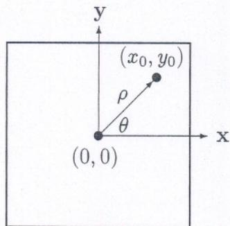
Figure 5.18: An enlarged view of the pixel at the center of the approximated function.  $(x_0, y_0)$  is the location of the edge as determined by Equations 5.41 and 5.42. This pixel will be marked as an edge pixel since the location of the edge falls within its boundaries.
