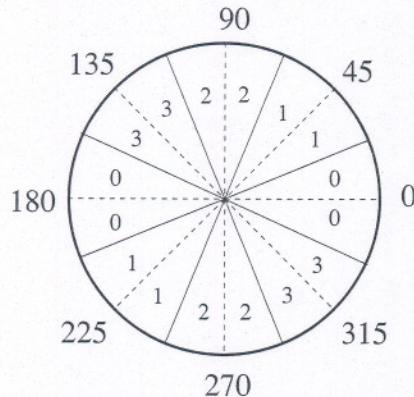
Figure 5.21: The partition of the possible gradient orientations into sectors for nonmaxima suppression is shown. There are four sectors, numbered 0 to 3, corresponding to the four possible combinations of elements in a  $3 \times 3$  neighborhood that a line must pass through as it passes through the center of the neighborhood. The divisions of the circle of possible gradient line orientations are labeled in degrees.
