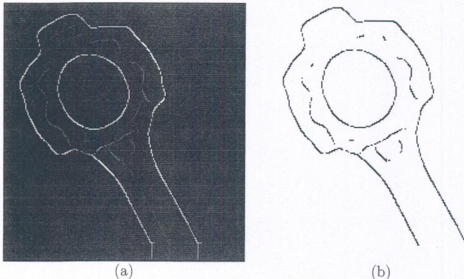
Figure 5.24: The result of edge detection applied to the test image from Figure 5.22. A  $31 \times 31$  Gaussian filter was used to smooth the image, followed by computation of the gradient approximation and then nonmaxima suppression. Part (a) displays the nonmaxima-suppressed result as a gray level image. Note how the large smoothing filter has rounded the edges. Part (b) plots the results to show all of the edge fragments.
