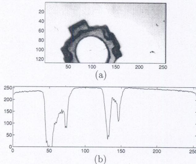
Figure 5.2: (a) The top half of the connecting rod image. (b) The profile of an ideal step change in image intensity is plotted to show that the edges are not perfectly sharp and the image is corrupted by noise. The plot is a horizontal slice through the circular portion of the connecting rod corresponding to the bottom edge of the partial rod image shown above.
