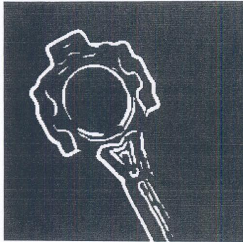
Figure 5.20: Edges obtained with facet model edge detector.
