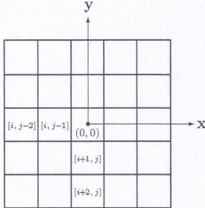
Figure 5.16: An example of the coordinate system for the facet model using a  $5 \times 5$  neighborhood. The continuous intensity function is approximated at every pixel location *only* within this neighborhood. The array indices are marked on the pixels for clarity. Note that pixel  $[i, j]$  lies in the center of the neighborhood.
