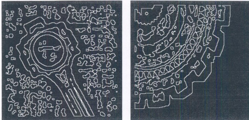
Figure 5.13: Results of the Laplacian of Gaussian edge detector.
