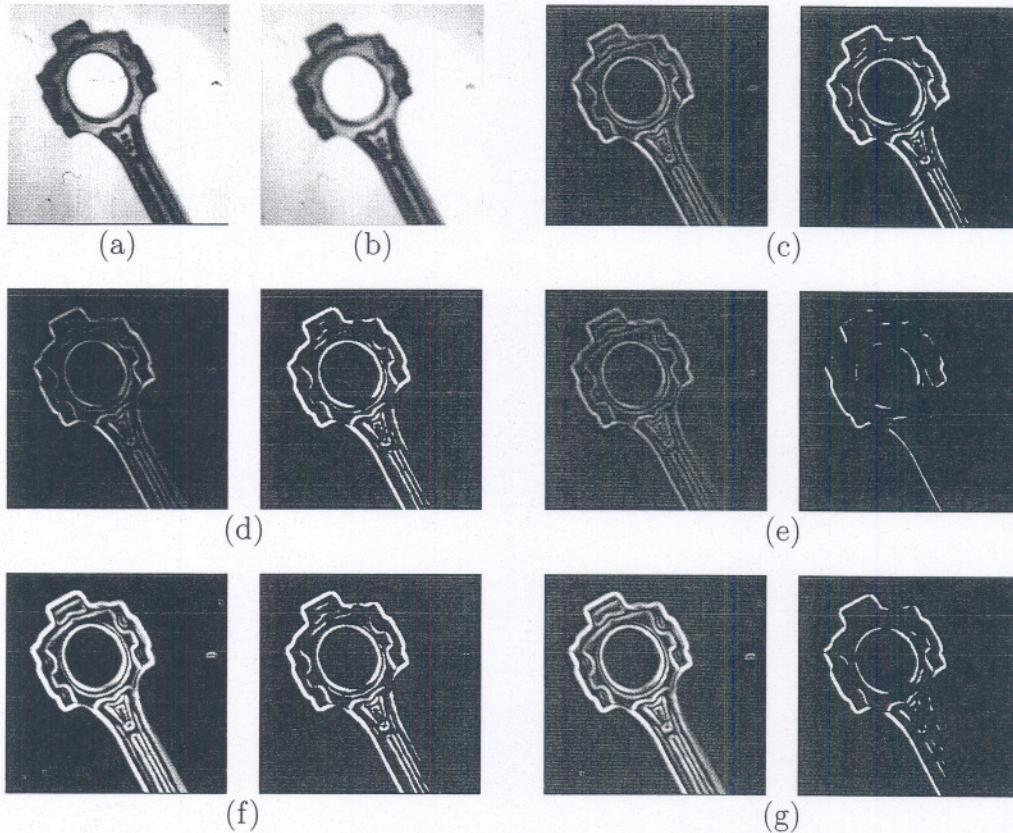
Figure 5.4: A comparison of various edge detectors. (a) Original image. (b) Filtered image. (c) Simple gradient using  $1 \times 2$  and  $2 \times 1$  masks,  $T = 32$ . (d) Gradient using  $2 \times 2$  masks,  $T = 64$ . (e) Roberts cross operator,  $T = 64$ . (f) Sobel operator,  $T = 225$ . (g) Prewitt operator,  $T = 225$ .
