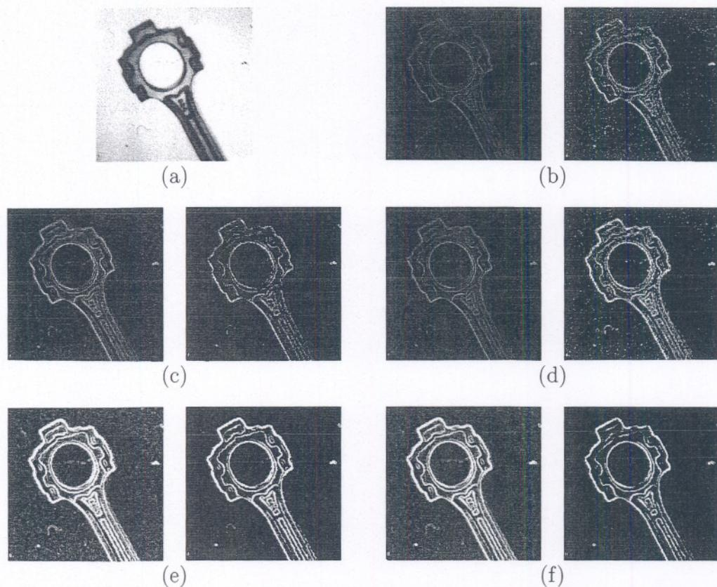
Figure 5.7: A comparison of various edge detectors on a noisy image without filtering. (a) Noisy image. (b) Simple gradient using  $1 \times 2$  and  $2 \times 1$  masks,  $T = 64$ . (c) Gradient using  $2 \times 2$  masks,  $T = 128$ . (d) Roberts cross operator,  $T = 64$ . (e) Sobel operator,  $T = 225$ . (f) Prewitt operator,  $T = 225$ .
