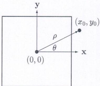
Figure 5.19: An enlarged view of the pixel at the center of the approximated function. This pixel will *not* be marked as an edge pixel since the location of the edge does not fall within the pixel boundaries.
