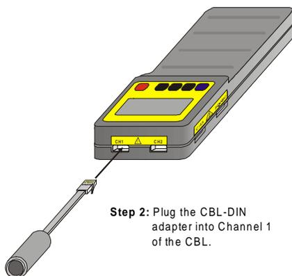
**Step 2:** Plug the CBL-DIN adapter into Channel 1 of the CBL.
