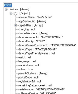
FIGURE 16-11 A query of the device information provides the name of the device, ID, customer ID, and serial number.
