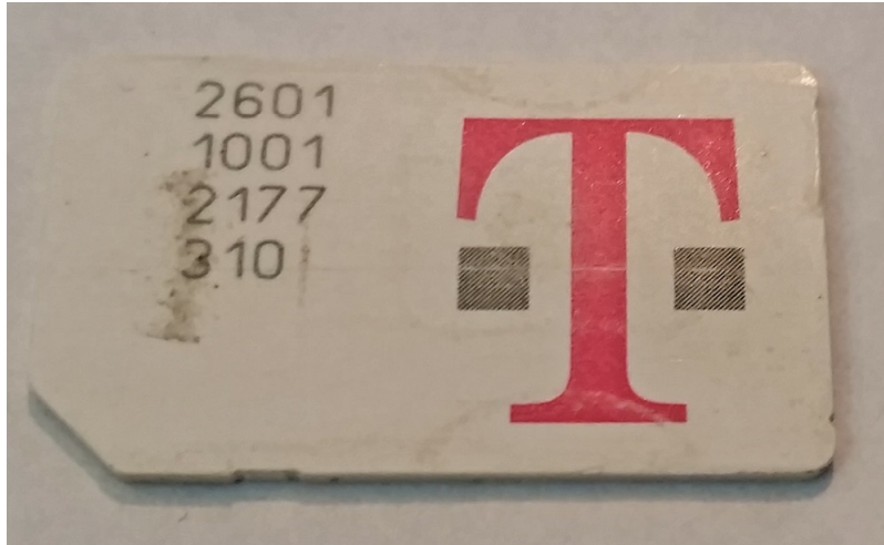
FIGURE 11-5 UICC exterior with a visible ICCID
