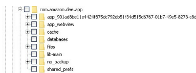
FIGURE 16-5 Folder structure of Alexa app within a Samsung SM-G900T running 5.11 Android
