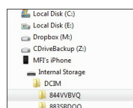
FIGURE 8-1 File system view of an iOS device connected as a PTP device—DCIM (Digital Camera Image) folder is available
