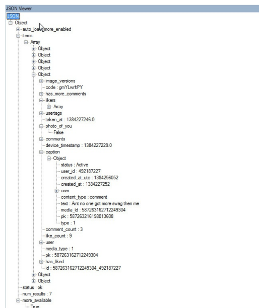
FIGURE 13-40 JSON file from Instagram's fsCachedData folder decoded into a readable format in Notepad++ with the JSON Viewer plug-in
