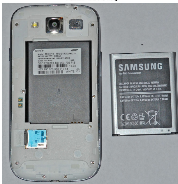
FIGURE 10-3 The serial numbers of the device should be clearly visible, along with the memory card still in place.
