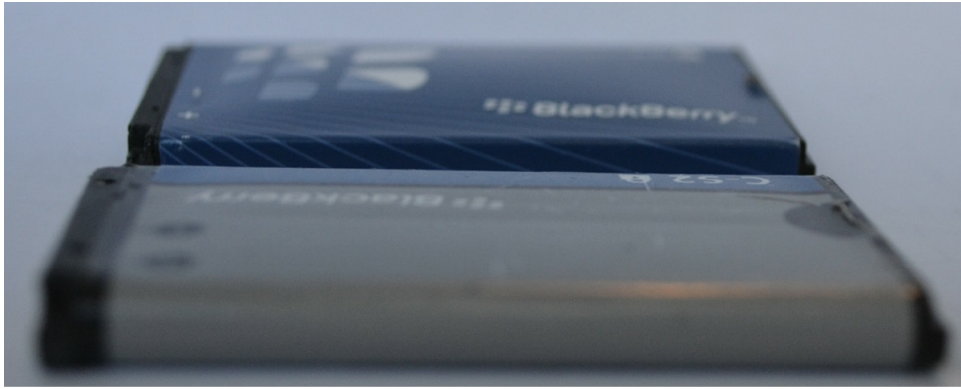
FIGURE 10-4 A normal battery (front) and a bloated battery (back). The middle of the back battery is distended and could explode, causing damage to the evidence and possibly the examiner.
