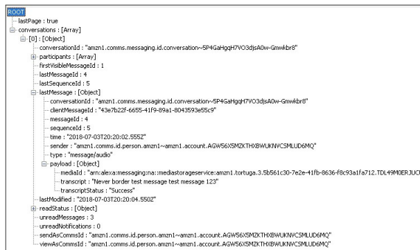
FIGURE 16-10 Results shown in Notepad++ with JSON viewer of messages from the Alexa Cloud
