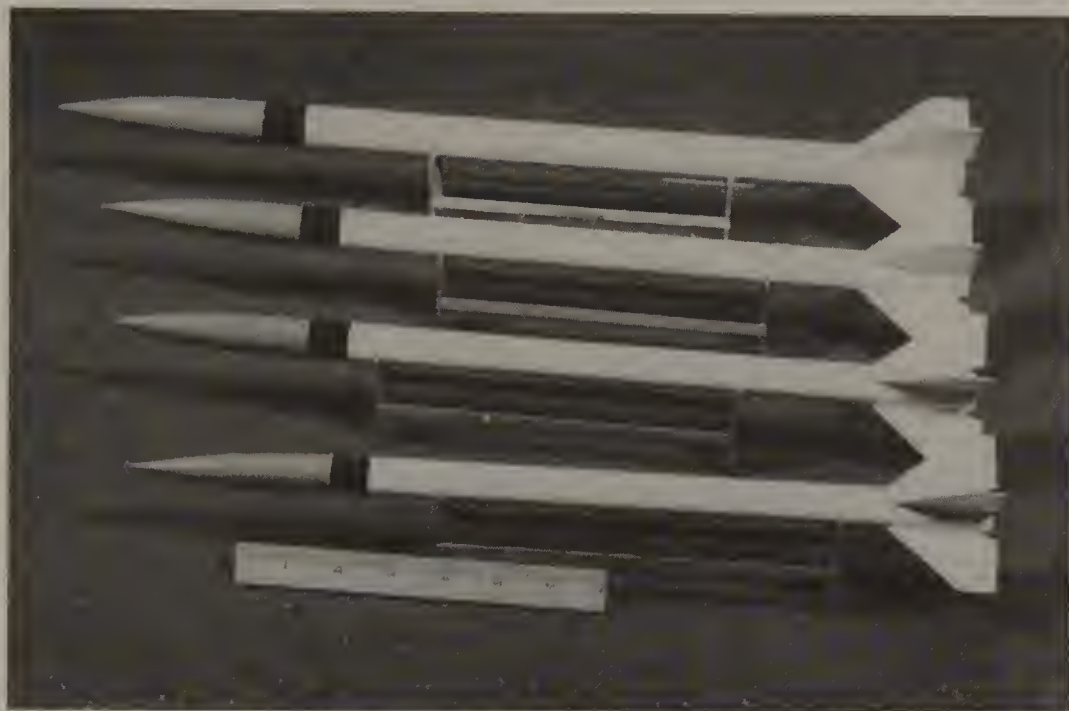
FIGURE 16-8 Building a scale model in a variety of different scales or sizes with body tubes of different diameters will help you get a good scale model that flies well. The author built these four I.Q.S.Y. Tomahawks in different scales to determine the best size.
