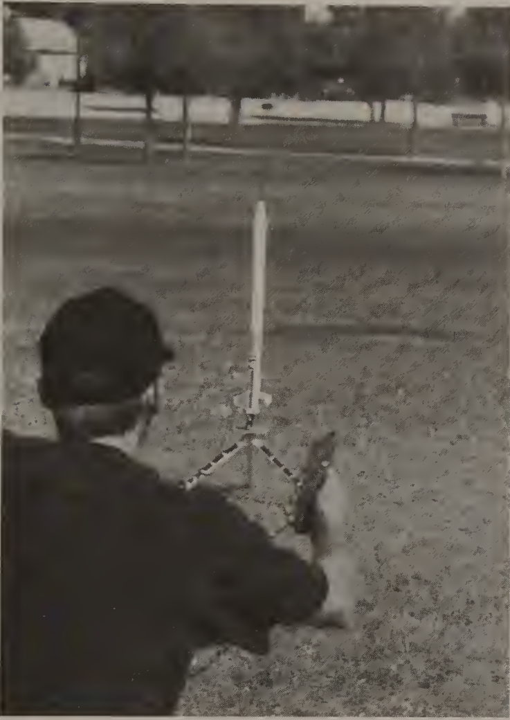
FIGURE 6-1 A model rocket is always launched by controlled electrical means using a launch pad and an electrical ignition system.
