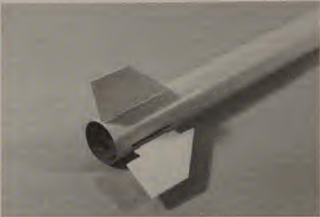
FIGURE 14-3 Through-the-wall fin attachment. The tab on the fin goes through the slot in the body tube and is bonded to the inner motor tube to provide added strength to withstand the forces created by higher airspeeds.
