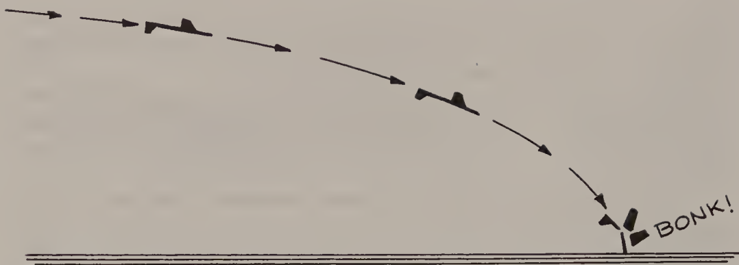
FIGURE 13-21 Nose-heavy gliding flight.
