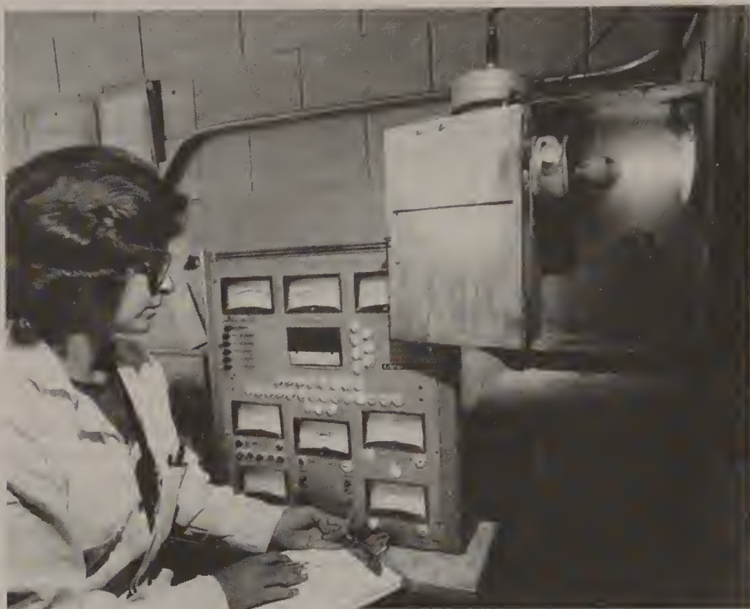
FIGURE 5-6 Static testing a model rocket motor to determine its performance. Manufacturers have developed complex electronic testing equipment to ensure high product reliability. (Estes Industries, Inc. photo.)
