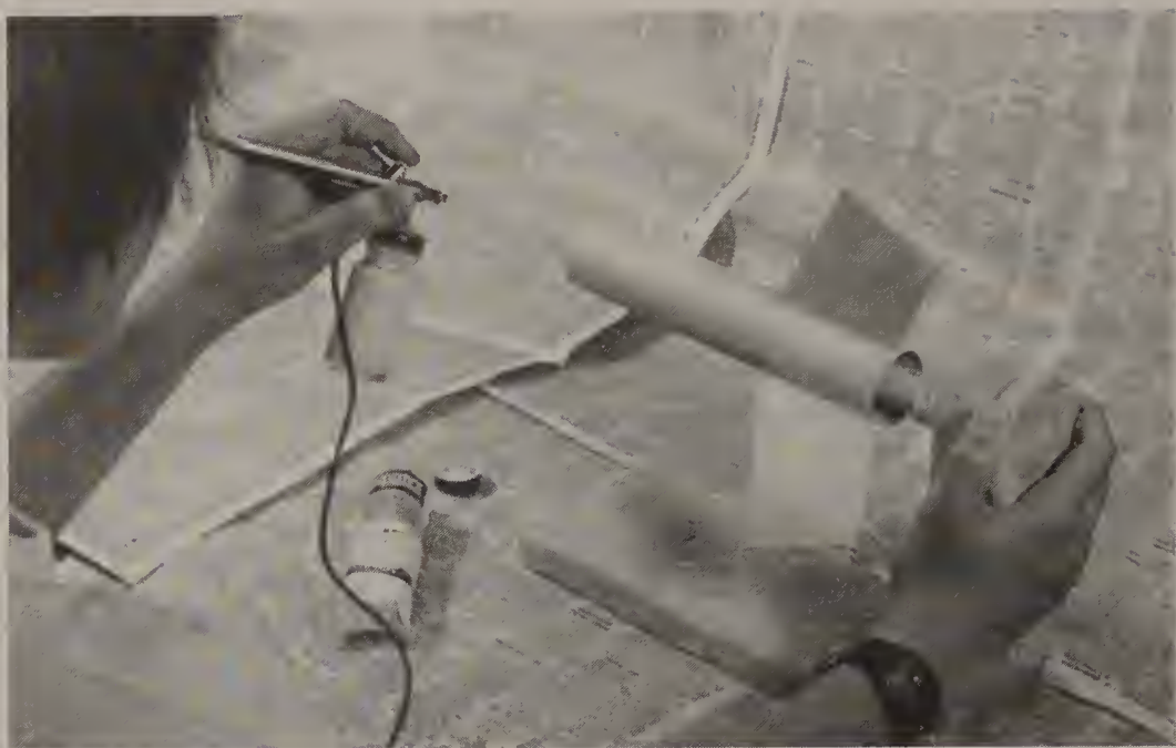
FIGURE 4-13 A hobby airbrush provides a beautiful, even coat of paint and is well worth the expense. Be sure to use lots of newspaper to prevent the overspray from getting everywhere.
