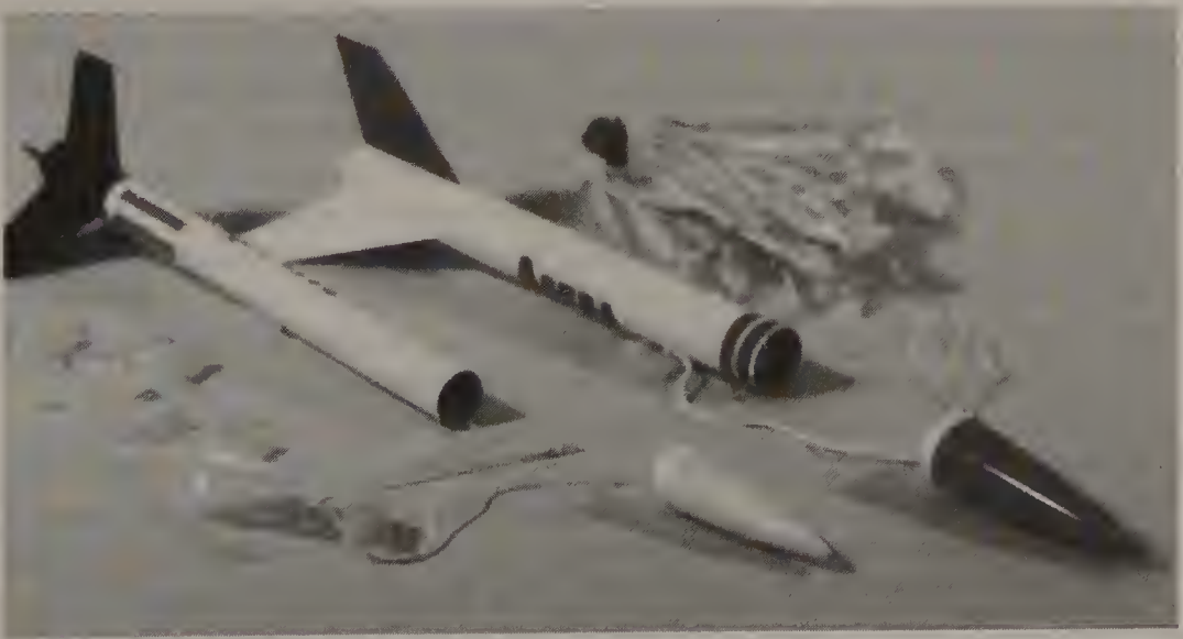
FIGURE 4-11 Two model rockets: one with a streamer for recovery and the other with a plastic parachute for a slower descent.
