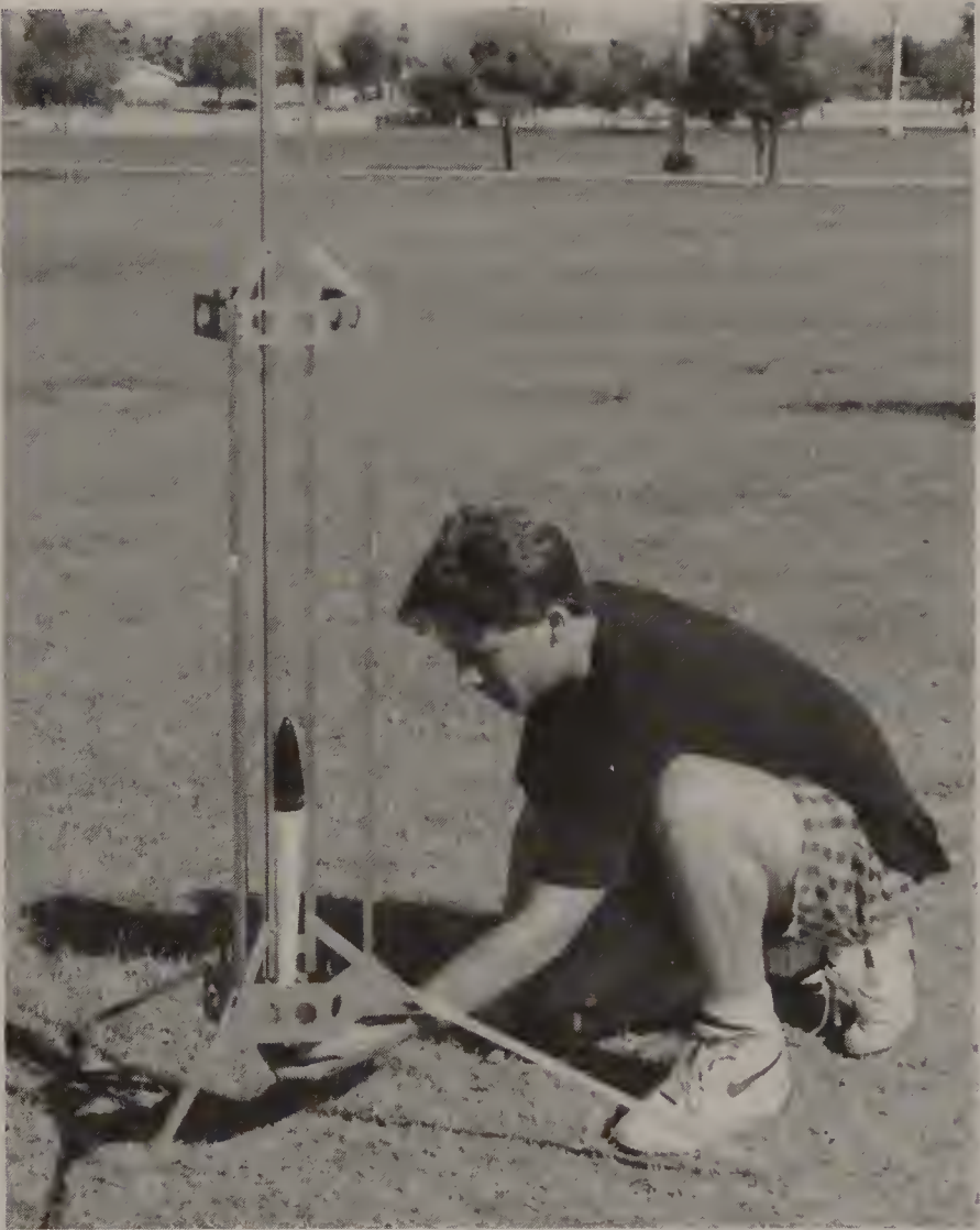
FIGURE 7-7 A tower launcher such as this one from Balsa Machining can be adjusted to accommodate models of different diameters. A tower eliminates the need for a launch lug and is stiffer than a standard rod for launching heavy models.
