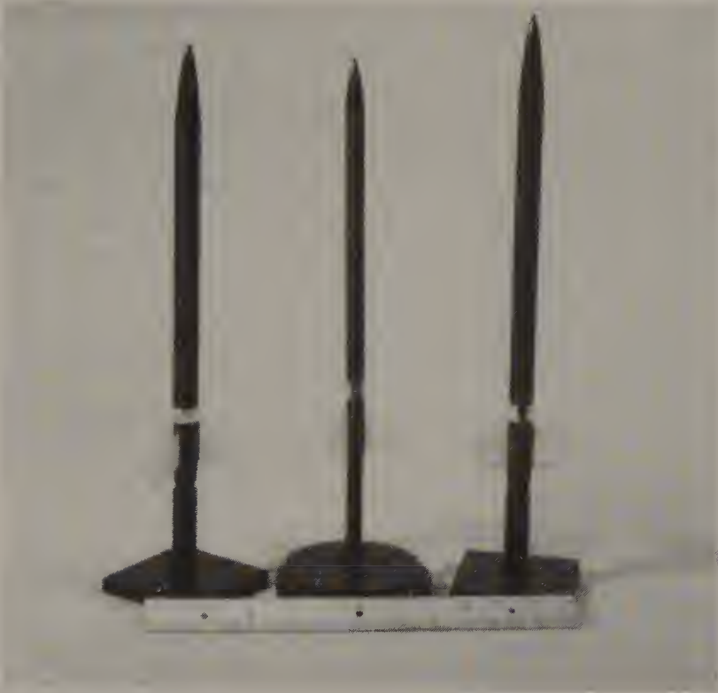
FIGURE 10-15 Some low-drag, high-performance contest model rockets. Fins are made from a very thin, semitransparent fiberglass sheet.
