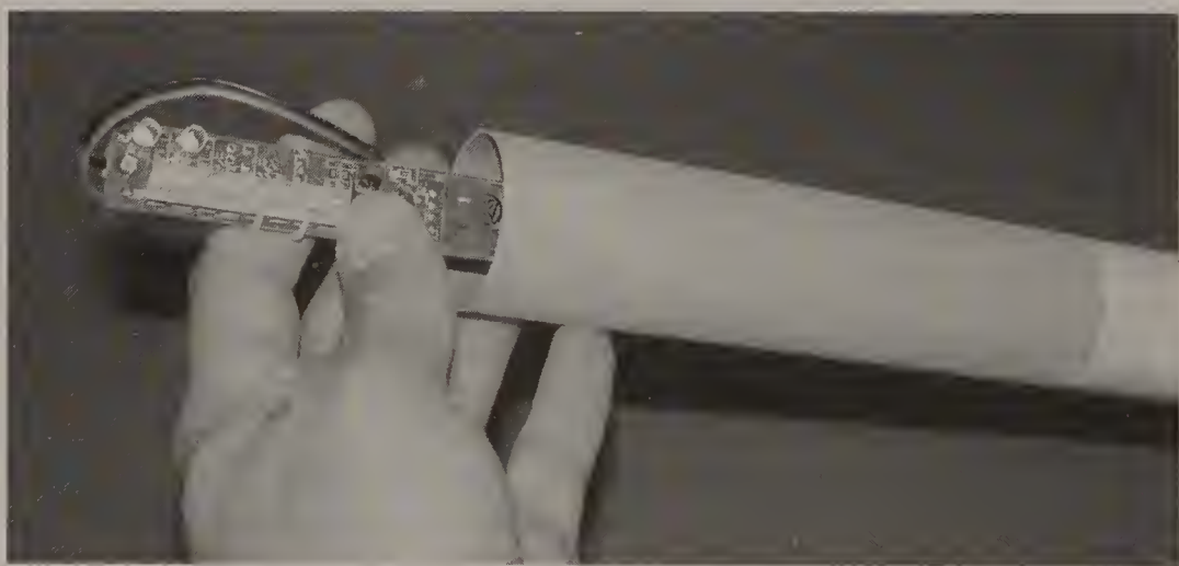
FIGURE 15-7 The G-Wiz LC standard flight computer uses proprietary firmware algorithms to determine the key events in a rocket's trajectory such as launch, booster burnout, sustainer burnout, coast, apogee, and low altitude.
