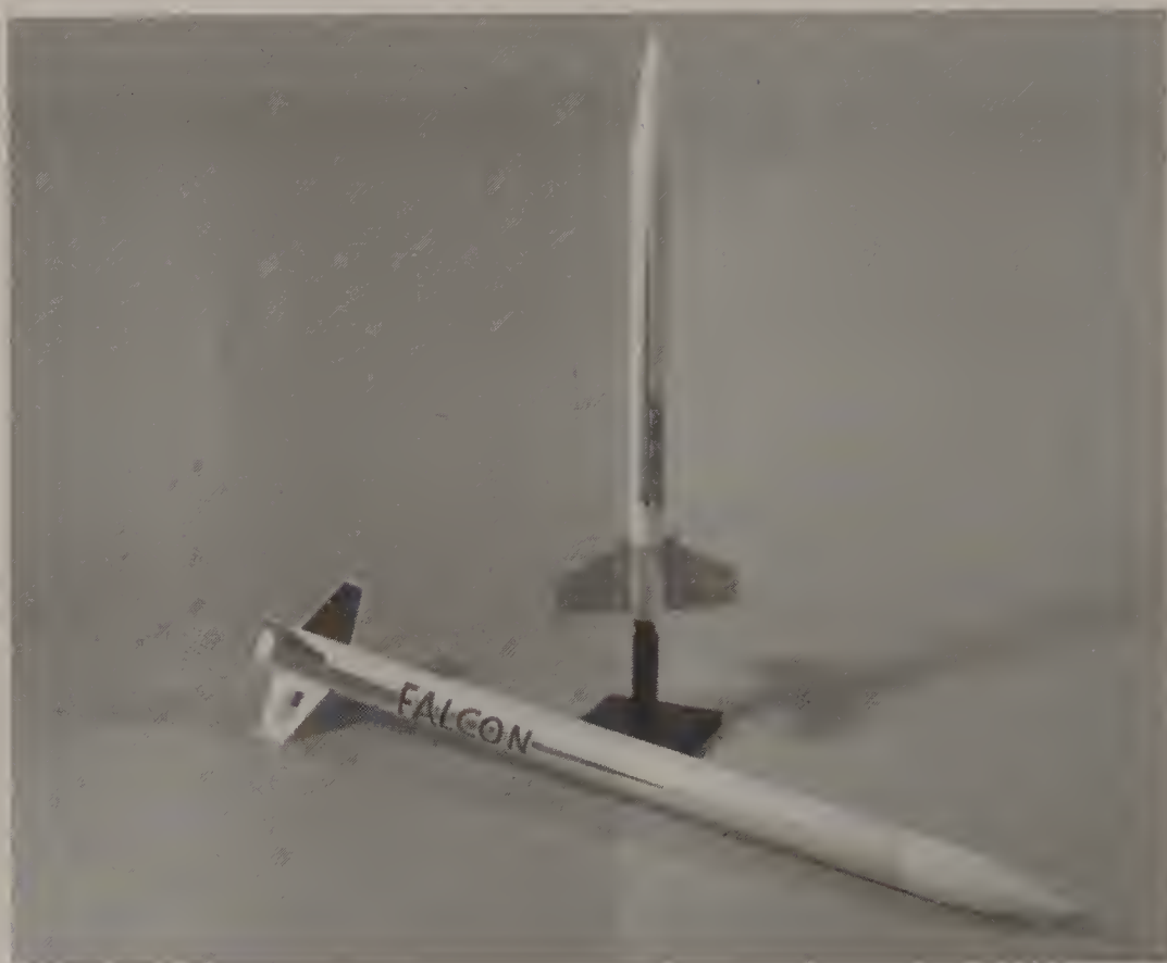
FIGURE 2-2 Two beginners' model rockets are the Quest Tracer (upright) and the Quest Falcon (horizontal). Both have plastic noses and fin units, color-coded parts, and no need for painting.
