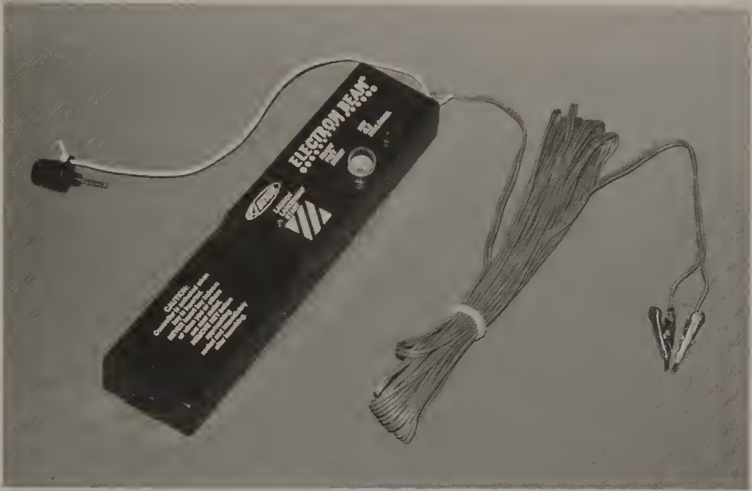
FIGURE 6-3 A typical commercial electrical launch controller with internal size AA alkaline penlight batteries for use with Estes and Quest igniters. Note the safety key and continuity check light.
