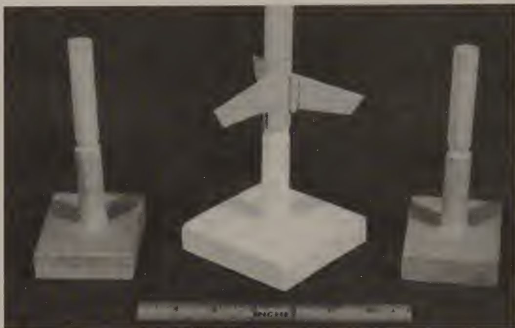
FIGURE 3-5 The workshop spike can be made from wood or plastic. It is designed to hold the model vertically.
