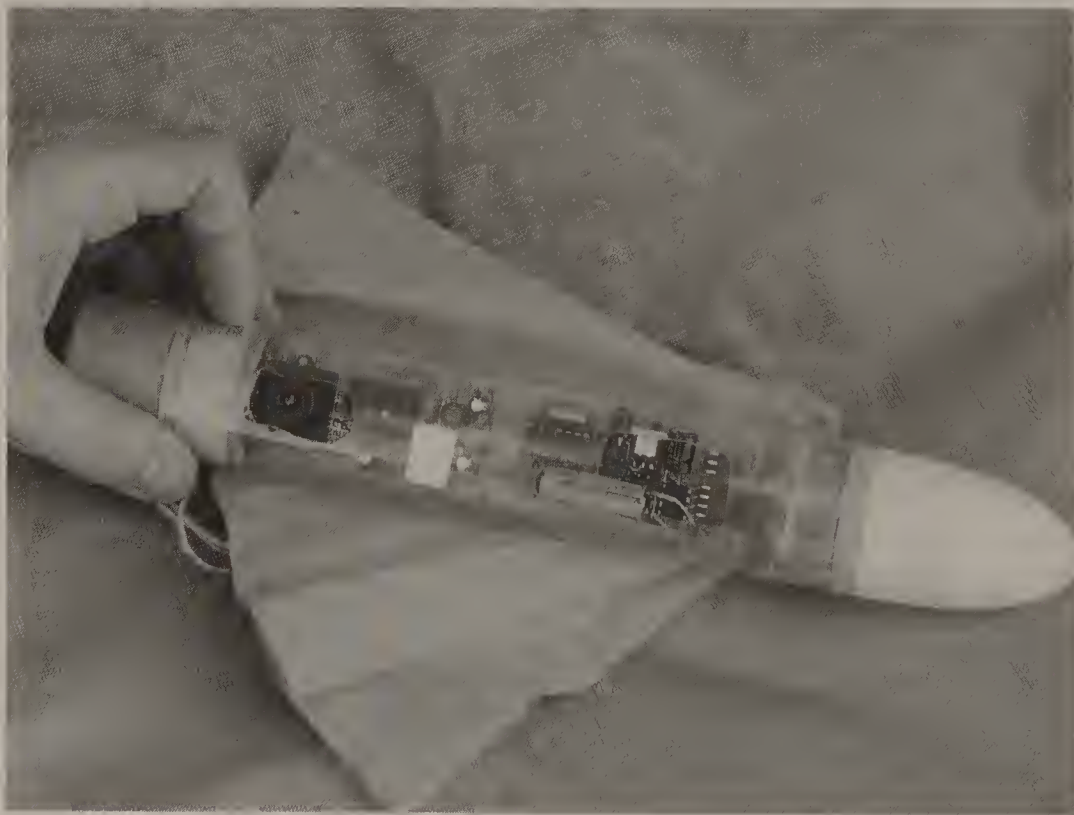
FIGURE 15-5 NAR member Bob Kaplow configured a clever conversion of a small digital LCD Pencam. Pictures are downloaded after flight via a USB cable. (Photo by Ric Gaff.)
