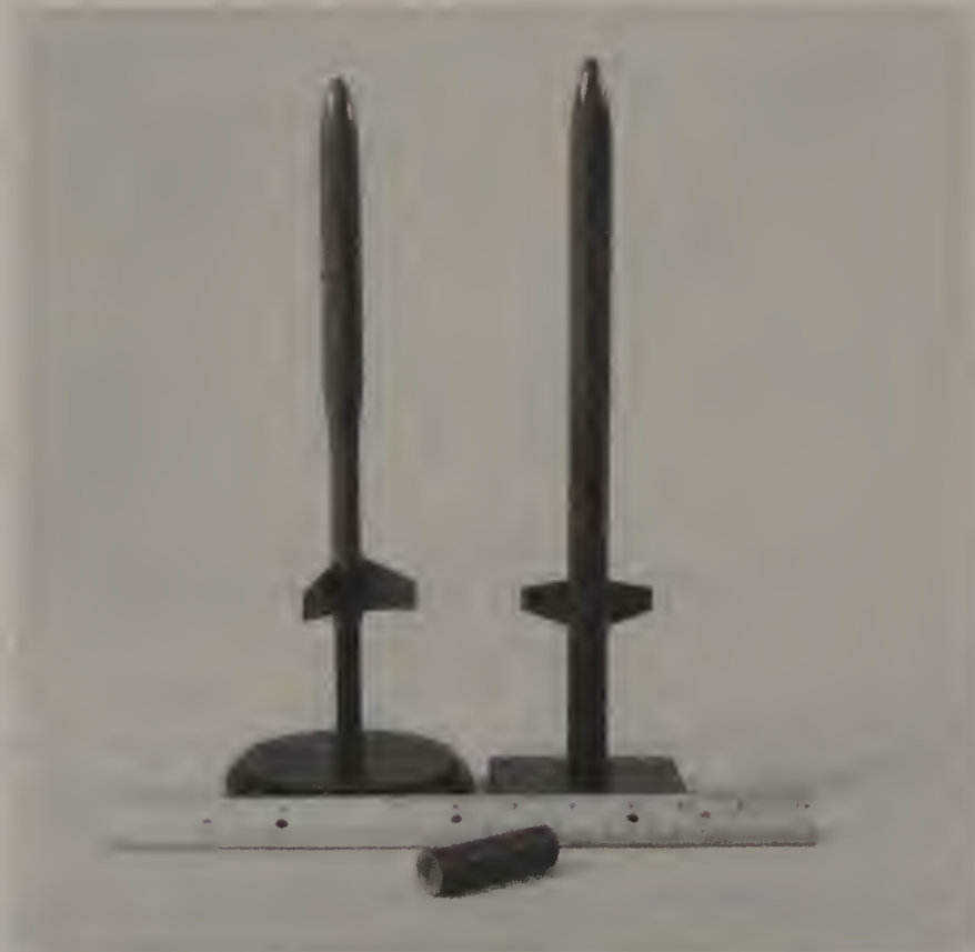
FIGURE 15-2 Two different contest models for the NAR Payload event. The standard payload is the black tube on the lower right.
