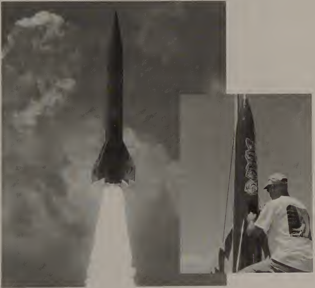
FIGURE 20-3 This 3X scaled-up Sumo was built by Dirk and Eric Gates. The rocket is powered by a total of four M motors. Inset photo: Eric is installing a digital video camera prior to launch at LDRS-21. (Photo by Gary Rosenfield.)
