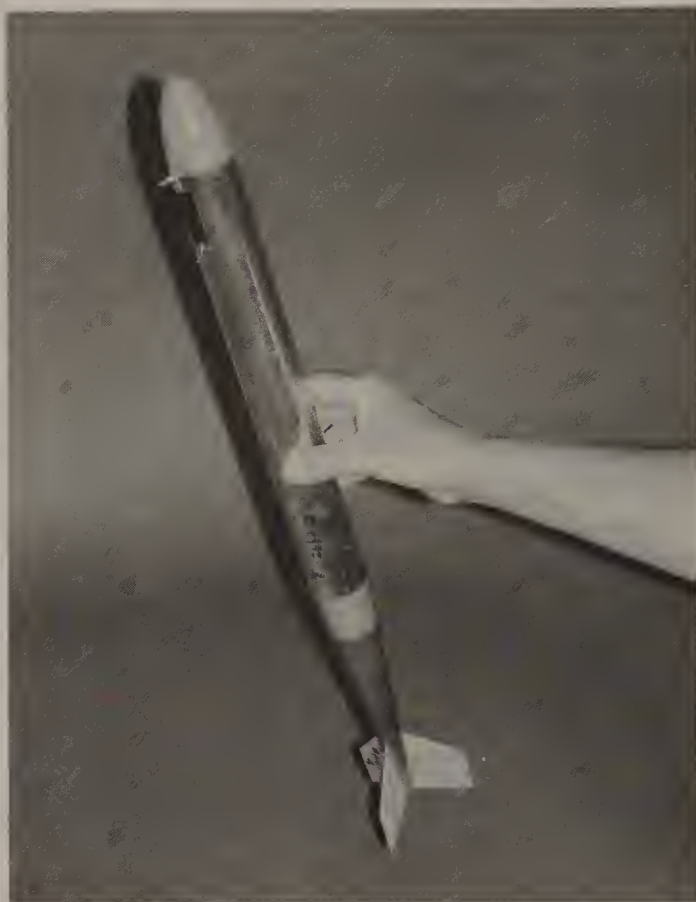
FIGURE 19-4 Model rockets used in international competition are very technically advanced. This 40-mm S3B parachute duration model is constructed from hand-layed-up fiberglass and epoxy. The model is wrapped in a silver reflective Mylar to improve visibility and colored tissue to reduce porosity of the fiberglass weave. It uses a micro-dethermalizer (DT) to bring the model down just after the 7-minute maximum flight time. It was flown in the 14th World Spacemodeling Championships in the Czech Republic by U.S. team member Mark Petrovich.
