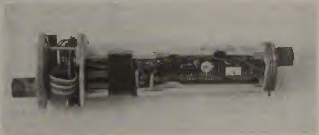
FIGURE 15-9 AED Electronics R-DAS mounted on its payload bay carrier. (Photo by Ken Horst.)
