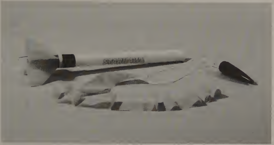
FIGURE 12-3 A streamer recovery model rocket has a paper or plastic streamer attached to the nose base or to the shock cord near the nose.
