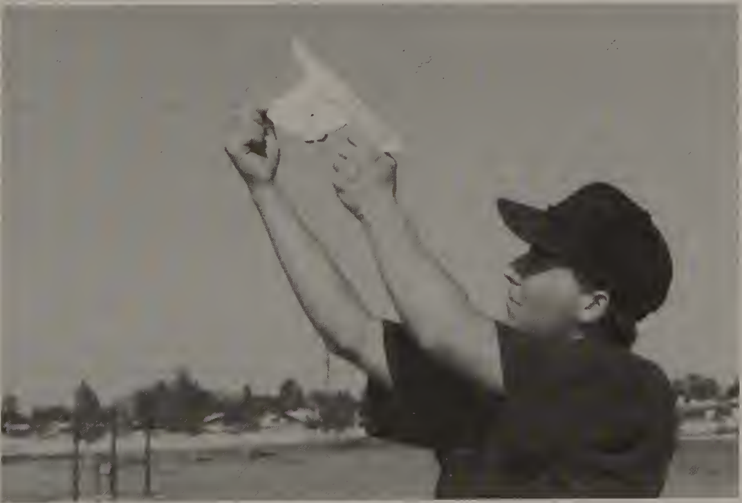
FIGURE 17-4 The Quest SkyScope is an inexpensive and simple elevation-angle-only tracking device.
