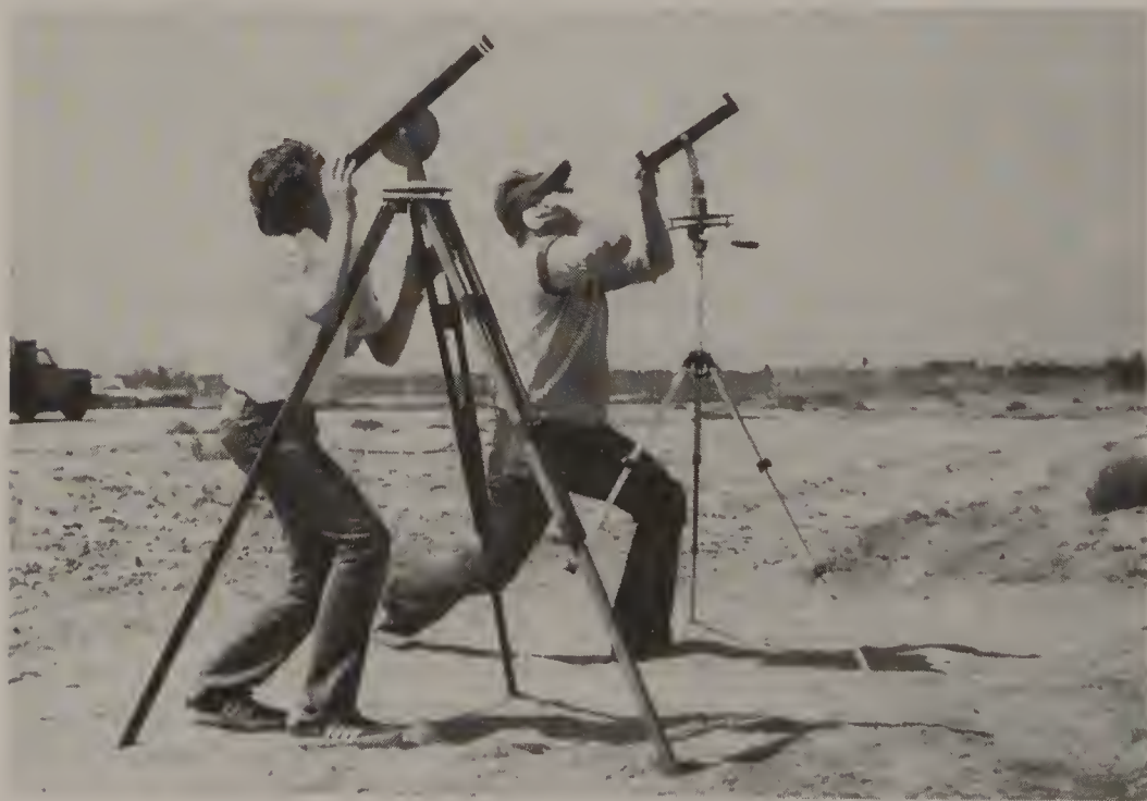
FIGURE 17-3 Model rockets can be tracked in flight with very simple equipment to obtain a definite figure for achieved altitude. Here, in national competition, two trackers are used at a station, one as a backup for the other.
