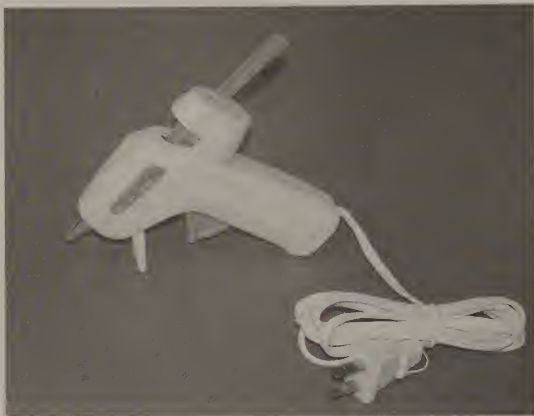
FIGURE 3-16 A craft hot melt glue gun is often used by teachers or youth group leaders during a group building session. The hot melt glue sets fast but gives students ample time to check their final fin alignment before setting.
