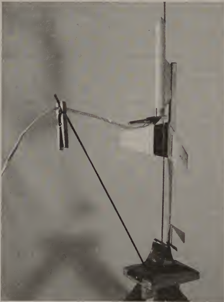
FIGURE 13-23 An umbilical mast installed on a launch pad to support the ignition wires and prevent them from fouling the tail of the B/G at liftoff.
