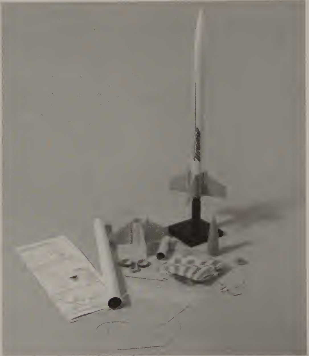
FIGURE 1-3 This typical model rocket, the Quest Tracer, is shown here in kit and assembled forms. It uses a plastic nose and tail fin unit, paper body, and parachute recovery.
