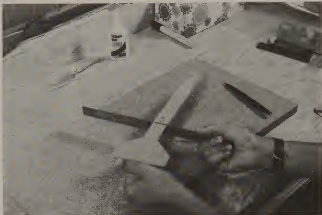
FIGURE 9-8 Checking the stability of a model rocket using a cardboard cutout of a side view of the model, thus locating its center of lateral area.
