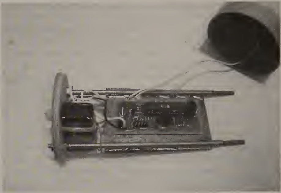
FIGURE 20-1 Electronics are commonly used to deploy recovery systems in high-power rocketry. This altimeter is a Missileworks RRC2 mounted on an electronics bay board cut by Precision G10.
