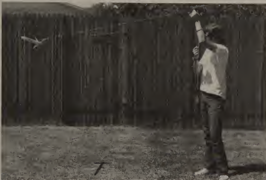
FIGURE 9-7 The easiest way to determine the stability of a model rocket is to conduct a swing test.
