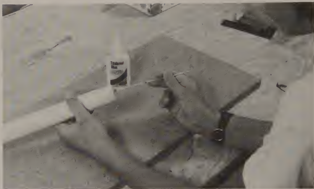
FIGURE 3-14 A cotton swab can be used to apply glue to the inside of a body tube. Mark the swab stick to indicate how far into the tube to apply the glue.
