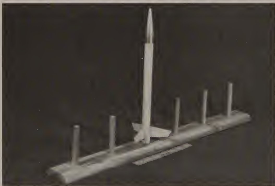
FIGURE 3-6 A spike row is a line of spike dowels on a single board for holding several models vertically.
