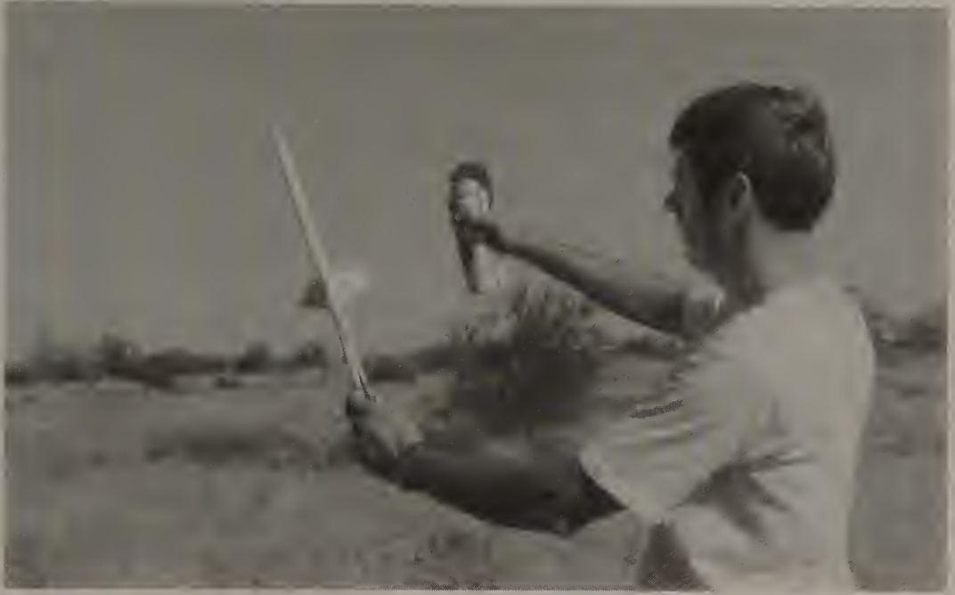
FIGURE 3-7 A paper painting wand is made from a section of newspaper rolled up and stuck into the rear end of the body tube. It keeps you from painting your hand when spray painting a model rocket.
