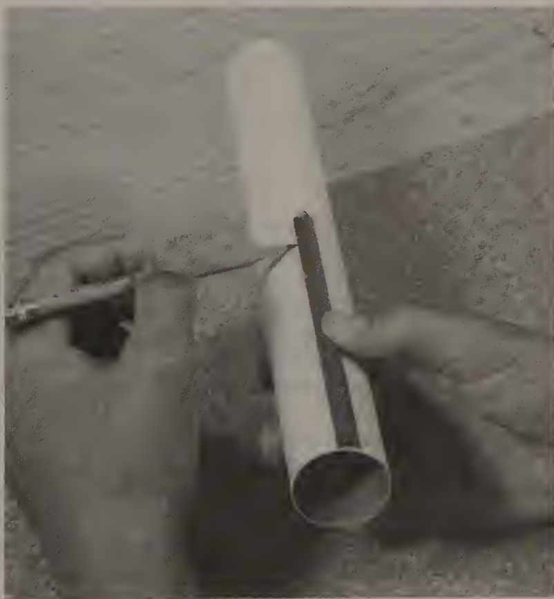
FIGURE 3-11 A small metal angle laid against the side of a body tube permits a straight line to be drawn down the tube for positioning the fins.
