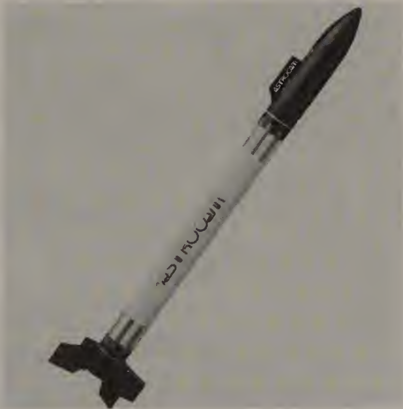
FIGURE 15-4 The Estes AstroCam 110 camera rocket takes a single color photo on each flight using Kodacolor 110 film. (Estes Industries, Inc., photo.)
