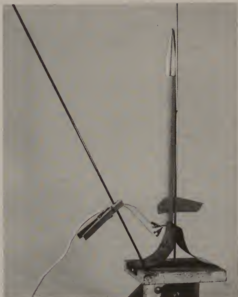
FIGURE 7-3 An umbilical mast and clothespin support the weight of the electrical leads and prevent igniter pull-out.
