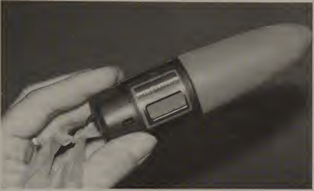
FIGURE 17-1 The Estes MaxTrax capsule is an electronic timer that times the fall of the capsule from apogee, then calculates the altitude.
