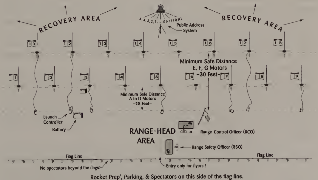
FIGURE 18-2 The layout of the range-head area of a model rocket range equipped to fly up to G motors. (Drawing by Ed LaCroix.)
