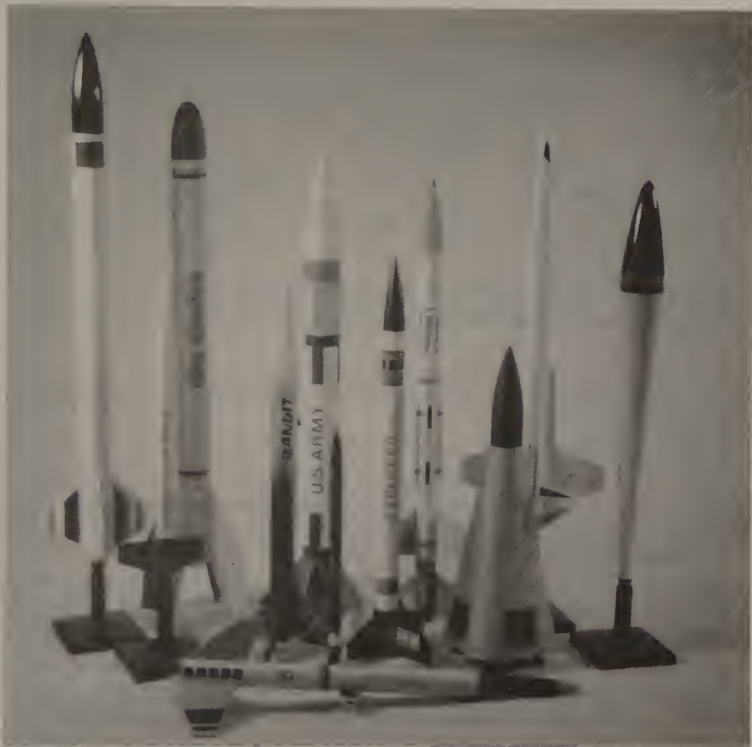
FIGURE 9-1 The size and shape of model rockets determine the air drag they will encounter in flight. Some shapes have less drag than others.
