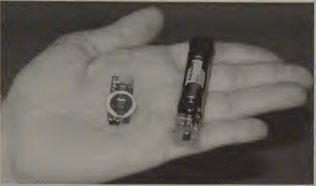
FIGURE 15-8 Two of the smallest altimeters available. On the left is the Altimate 1 from BonNova. It weighs 4.5 grams with battery and can record altitudes up to 30,000 feet AGL. On the right is the Adept Instruments Model A1. It records altitudes up to 3,000 feet AGL.
