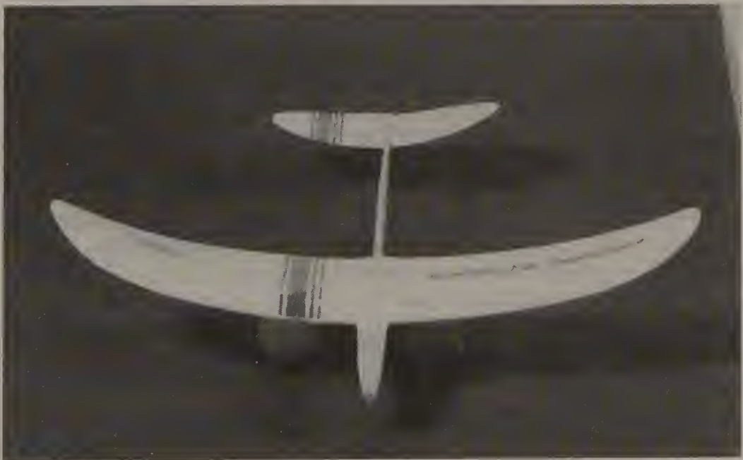
FIGURE 13-11 Elliptical dihedral of a wing.
