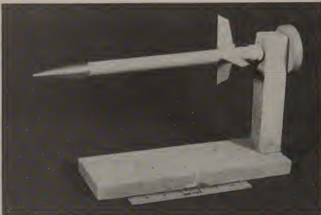
FIGURE 3-8 A rotating spike holds a model rocket horizontally so that it can be turned to spray paint all sides of it.
