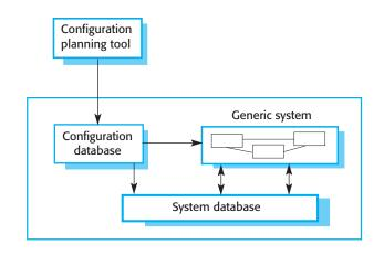
**Figure 15.11** Deployment-time configuration
