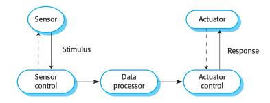
Figure 21.3 Sensor and actuator processes
