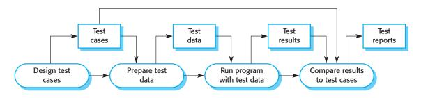
Figure 8.3 A model of the software testing process
