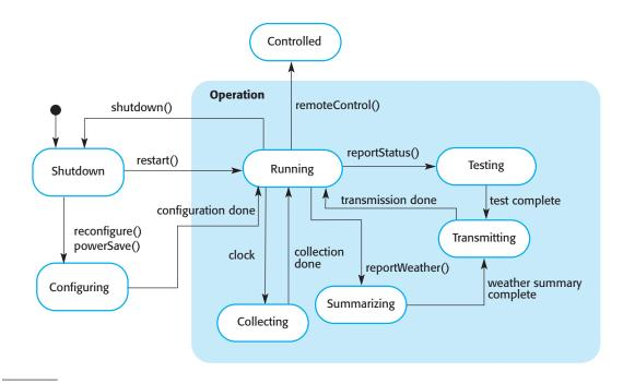
Figure 7.8 Weather station state diagram
