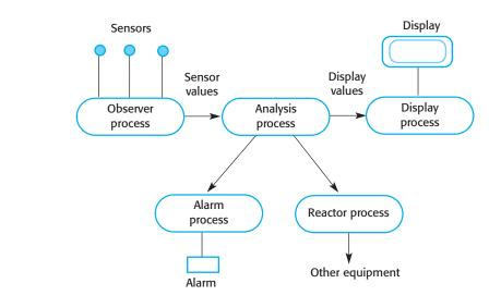
**Figure 21.7** The Observe and React process structure
