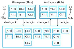
Figure 25.5 Check-in and check-out from a centralized version repository
