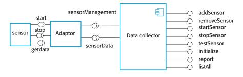
Figure 16.12 An adaptor linking a data collector and a sensor
