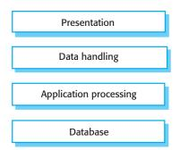
**Figure 17.6** Layered architectural model for client–server application
