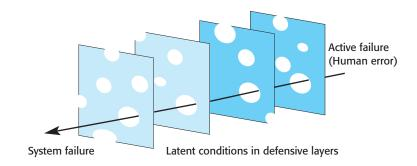
**Figure 14.6** Reason's Swiss cheese model of system failure
