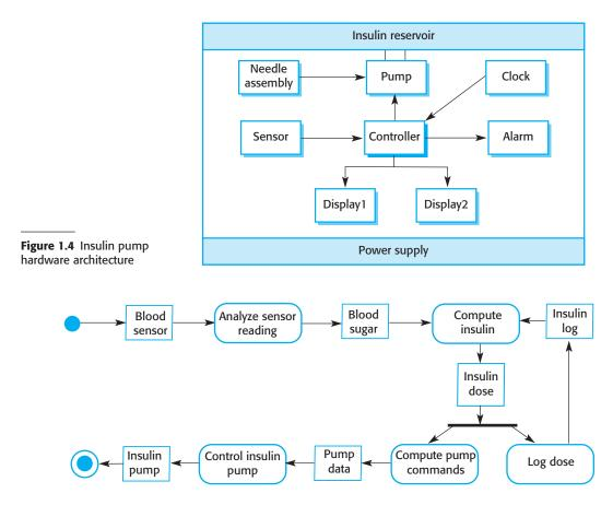
Figure 1.5 Activity model of the insulin pump ultimately, unconsciousness and death. In the long term, however, continual high levels of blood glucose can lead to eye damage, kidney damage, and heart problems.
