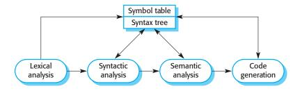
**Figure 6.22** A pipe and filter compiler architecture
