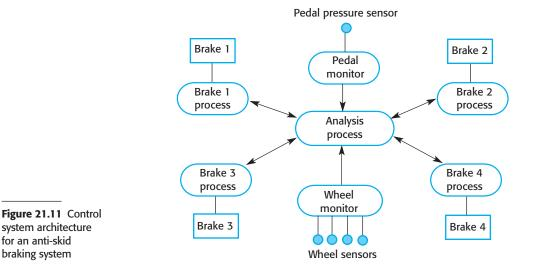
from the equipment's environment. For example, an anti-skid braking system in a car monitors the car's wheels and brake system (the system's environment). It looks for signs that the wheels are skidding when brake pressure is applied. If this is the case, the system adjusts the brake pressure to stop the wheels locking and reduce the likelihood of a skid.
