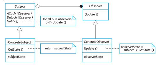
**Figure 7.12** A UML model of the Observer pattern
