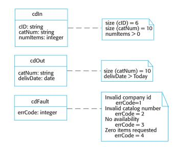
**Figure 18.12** UML definition of input and output messages
