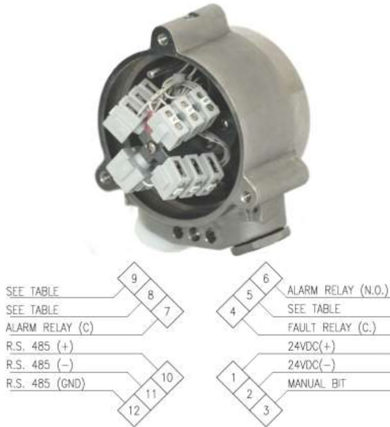
Figure 9: Wiring Terminals
