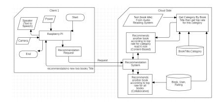
Figure 2: Block Diagram of recommendation system
