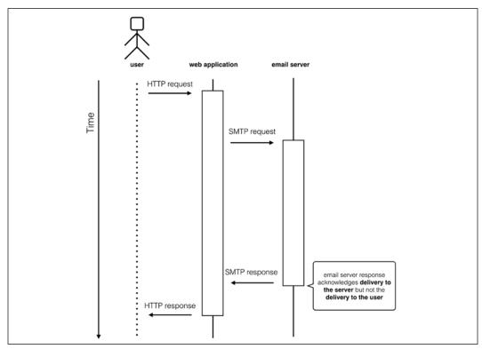
Figure 13.6: An example of synchronous email delivery in a web application
