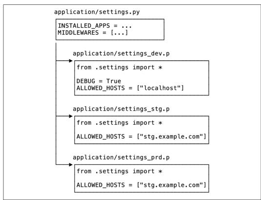
Figure 11.1: Typical layout of settings modules in many Django applications
