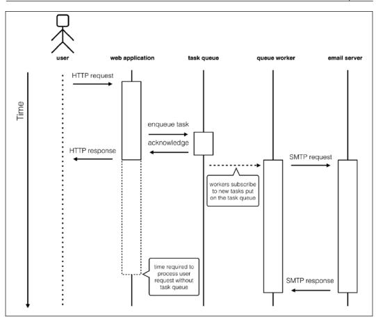
Figure 13.7: An example of asynchronous email delivery in a web application
