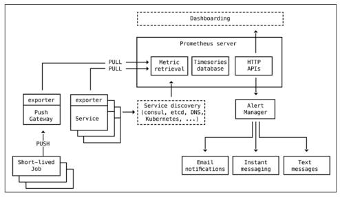
Figure 12.2: Architecture of a typical Prometheus deployment
