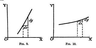
If the curve slopes up very gently, as in Fig. 10,  $\frac{dy}{dx}$  will be a fraction smaller than 1.
