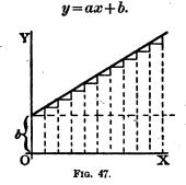
We know that here b represents the initial height of y when x=0, and that a, which is the same as  $\frac{dy}{dx}$ , is the "slope" of the line. The line has a constant slope. All along it the elementary triangles  $\int \frac{dy}{dx} \frac{dy}{dx}$ have the same proportion between height and base. Suppose we were to take the dx's and dy's of finite magnitude, so that 10 dx's made up one inch, then there would be ten little triangles like
