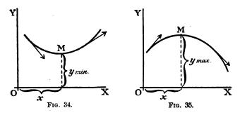
getting more and more upward. Clearly the change of slope as the curve passes through M is such that  $\frac{d^2y}{dx^2}$  is *positive*, for its operation, as x increases toward the right, is to convert a downward slope into an upward one.
