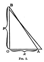
*AB*, of fixed length; and let y be the height it reaches up the wall. Now y clearly depends on x. It is easy to see that, if we pull the bottom end A a bit further from the wall, the top end B will come down a little lower. Let us state this in scientific language. If we increase x to x+dx, then y will become y-dy; that is, when x receives a positive
