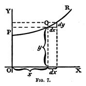
Let PQR, in Fig. 7, be a portion of a curve plotted with respect to the axes of coordinates OX and OY. Consider any point Q on this curve, where the abscissa of the point is x and its ordinate is y. Now observe how y changes when x is varied. If x
