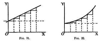
tion, as applied to curves,  $\frac{dy}{dx}$  means the *slope* of the curve. But what can  $\frac{d^2y}{dx^2}$  mean in this case? Clearly it means the rate (per unit of length x) at which the slope is changing—in brief, it is a measure of the curvature of the slope.
