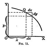
If a curve slopes downward, as in Fig. 11, dy will be a step down, and must therefore be reckoned of negative value; hence  $\frac{dy}{dx}$  will have negative sign also.
