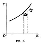
If a curve is sloping up at 45° at a particular point, as in Fig. 8, dy and dx will be equal, and the value of  $\frac{dy}{dx} = 1$ .
