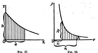
(4) Another example is afforded by the adiabatic curve of a perfect gas, the equation to which is  $pv^n = c$ , where p stands for pressure, v for volume, and n is of the value 1.42 (Fig. 58).
