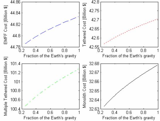
**Figure 11 Effect of varying the fraction of Earth's gravity on cost**
