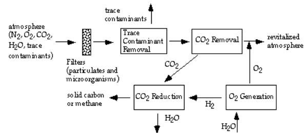
**Figure 4** Atmosphere control and supply<sup>9</sup>
