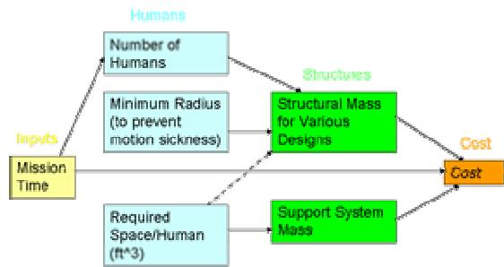
**Figure 2. Relationships between the various subsystems of the tool.**
