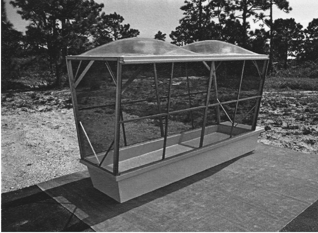
Figure 7.3 Miniature greenhouse structure with the base containing the nutrient solution that is periodically pumped into the gravel bed for rooting plants.
