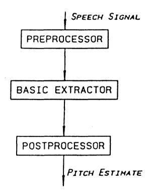
Figure 3.4 Block diagram illustrating the basic stages involved in speech fundamental frequency/period, estimation.
