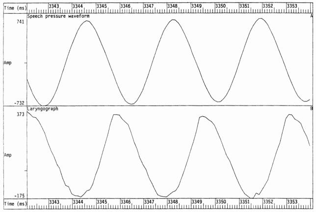
Figure 3.3 Temporally simple speech pressure waveform.
