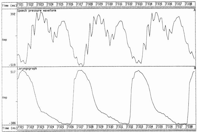
Figure 3.2 Speech pressure waveform exhibiting two peaks per fundamental period. The speech is shown in trace A. The corresponding laryngograph waveform in shown in trace B. This situation arises when the first formant coincides with the second harmonic in the excitation spectrum. This situation can lead to "doubling error" in simple fundamental period estimation algorithms. The speech is the vowel /I/ from a male subject.
