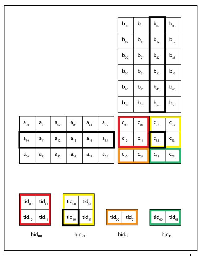
\_\_\_\_\_global\_\_ void MatrixMulKernel(float\* d\_M, float\* d\_N, float\* d\_P, int Width)
