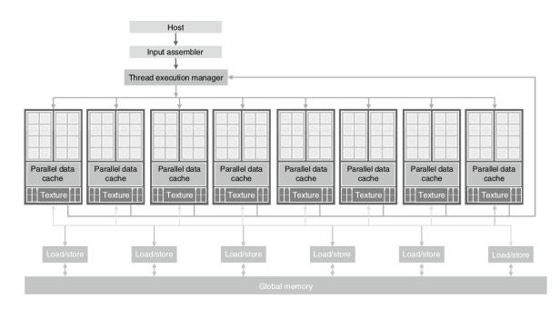
There are 16 streaming multiprocessors (SMs) in the above diagram. Each SM has 8 streaming processors (SPs). That is, we get a total of 128 SPs. Now, each SP has a MAD unit (Multiply and Addition Unit) and an additional MU (Multiply Unit). The GT200 has 240 SPs, and exceeds 1 TFLOP of processing power.
