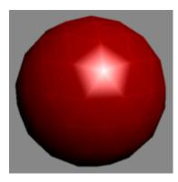
Let us now see shading using Gouraud shading. The triangle count is poor, and hence the poor performance of the specular highlight.
