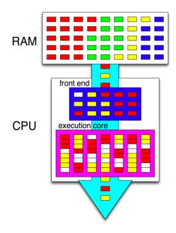
The pink box represents a single CPU core. The RAM contains instructions of 4 different programs, indicated by different colors. The CPU implements the SMT, using a technology similar to hyper-threading. Hence, it is able to run instructions of two different programs (red and yellow) simultaneously. White boxes represent pipeline stalls.
