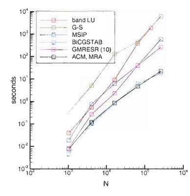
Figure 3.18: Time of computation at Re=0 for different size problems.
