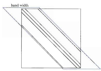
Figure 3.4: The draft of the 2D-5PF case with a band width painted in blue. It evolves the five diagonals.
