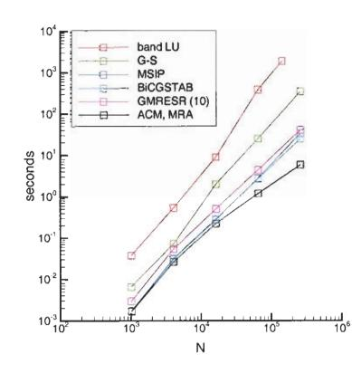
Figure 3.16: Time of computation at Re=100 for different size problems.
