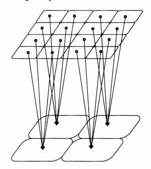
Figure 3.13: Restriction process over blocks of four grid points.
