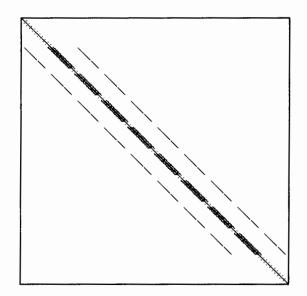
Figure 3.7: The kij ordering for a  $10 \times 10 \times 10$  case with 7-point formulation.
