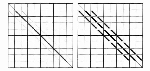
Figure 3.3: 3D-7PF (left) and 3D-19PF (right) for a  $10 \times 10 \times 10$  case. Each of these squares has  $100 \times 100$  entries.
