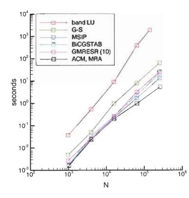
Figure 3.17: Time of computation at Re=10000 for different size problems.
