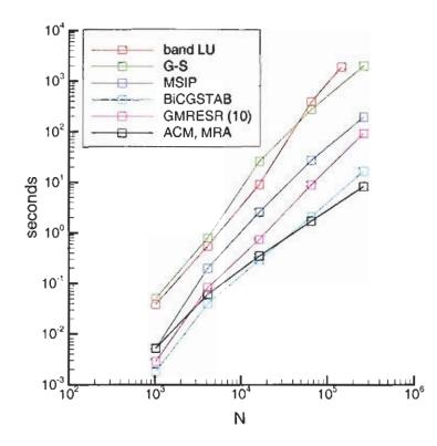
Figure 3.15: Time of computation at Re=0 for different size problems.
