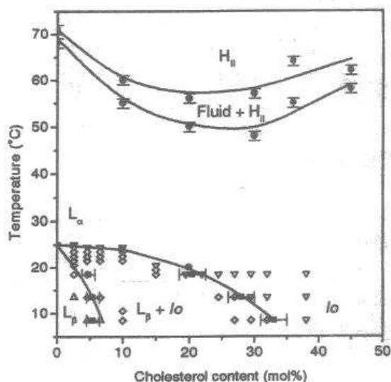
Figure 4.2: A partial phase diagram of POPE–cholesterol mixtures obtained from IR and NMR spectroscopy.  $H_{II}$  : inverted hexagonal phase,  $L_{\alpha}$  : fluid phase,  $L_{\beta}$  : gel phase,  $l_o$  : cholesterol–rich fluid phase [11].
