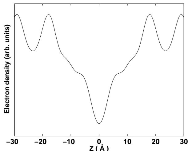
Figure 4.11: Transbilayer electron density profile of DLPE-cholesterol mixture ( $X_c = 30$  mol%,  $T = 6^\circ\text{C}$ ,  $\text{RH} = 98\%$ ). Peaks near  $\pm 20 \text{ \AA}$  and the trough at the center correspond to the head groups and terminal methyl groups of the hydrocarbon chains, respectively. Shoulder near  $\pm 10 \text{ \AA}$  are due to the presence of cholesterol.
