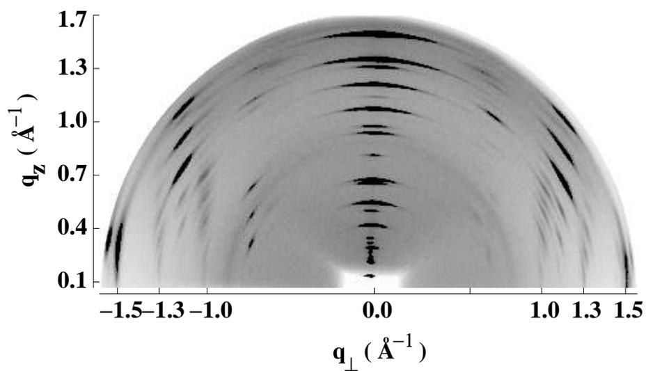
Figure 4.5: Diffraction pattern of a highly ordered phase of DLPE before heating to high temperatures.
