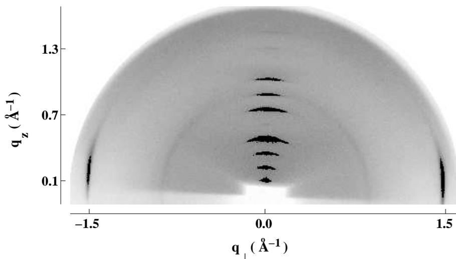
Figure 4.3: Diffraction pattern of the  $L_\beta$  phase of DLPE ( $T = 10^\circ\text{C}$ ,  $\text{RH} = 98\%$ ). The absence of chain tilt is indicated by the on-axis ( $q_z = 0$ ) wide angle reflections. The shadow at the bottom is due to absorption by the substrate. The diffuse ring near  $q = 0.7$  is due to the mylar windows of the sample chamber.
