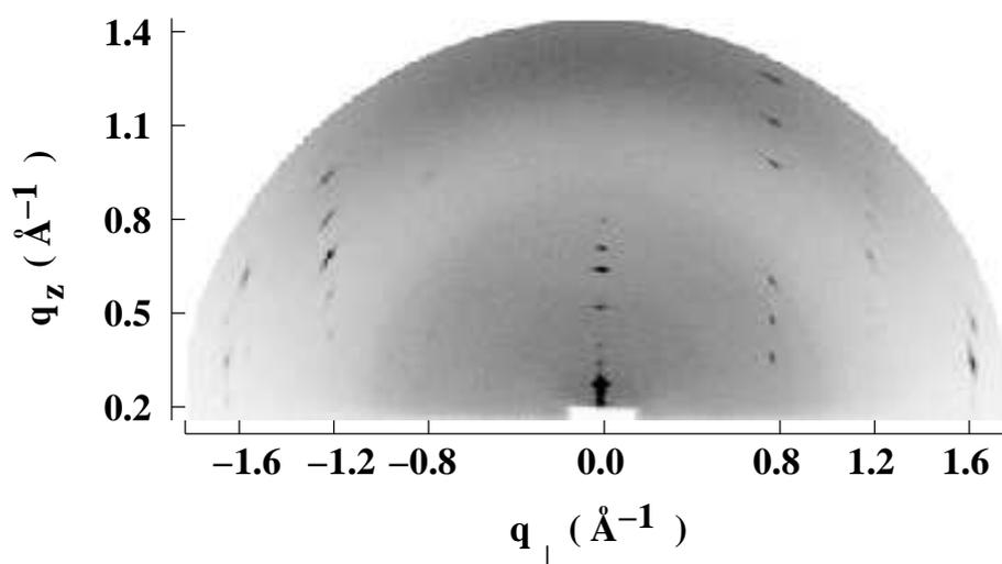
Figure 4.6: Diffraction pattern of a highly ordered phase of DLPE-cholesterol mixtures observed on cooling the sample from the  $L_\alpha$  phase.
