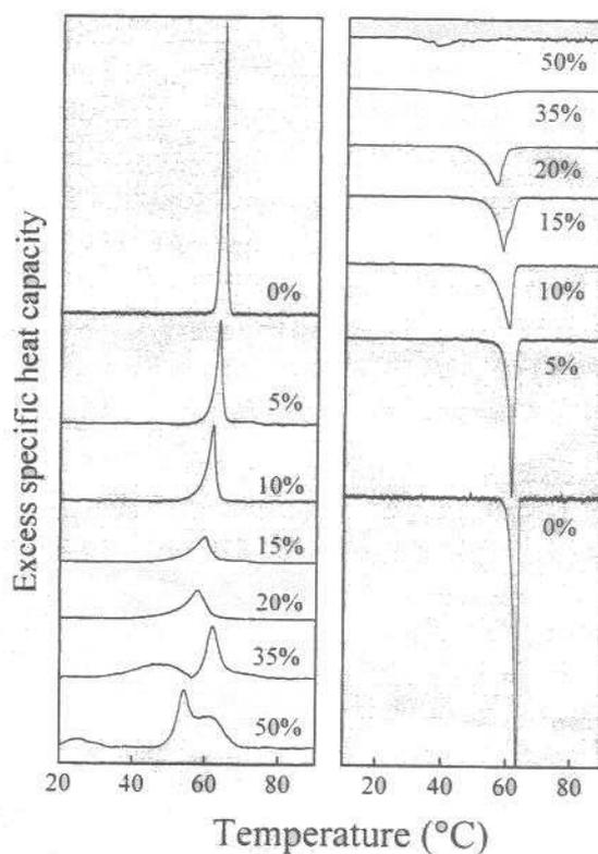
Figure 4.1: DSC thermograms of DPPE–cholesterol mixtures at various cholesterol concentrations as indicated by the labels on the curves, obtained during heating (left) and cooling (right). [2].
