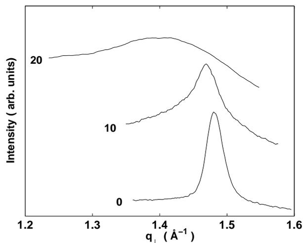
Figure 4.13: Wide angle reflections of DLPE bilayers at different cholesterol concentrations indicated by the labels on the curves ( $T = 20^{\circ}\text{C}$ ,  $\text{RH} = 98\%$ ).
