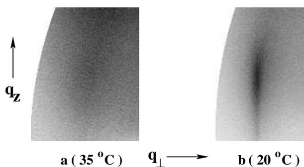
Figure 4.8: The wide angle reflections of DLPE-cholesterol mixture at  $X_c = 10$  mol% ( $d = 4.5 \text{ \AA}$  at  $35^\circ\text{C}$ ,  $d = 4.2 \text{ \AA}$  at  $20^\circ\text{C}$ ).
