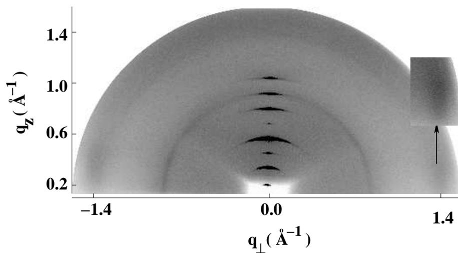
Figure 4.9: Diffraction pattern of the cholesterol-rich  $l_o$  phase ( $X_c = 20$  mol%,  $T = 10^\circ\text{C}$ ,  $\text{RH} = 98\%$ ). The inset is the wide angle reflection at a higher contrast. The diffuse ring near  $q = 0.7$  is due to the mylar windows of the sample chamber.
