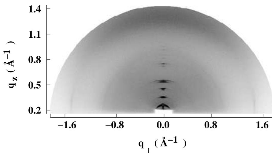
Figure 4.7: Diffraction pattern of a DLPE-cholesterol mixture showing the coexistence of the  $L_\beta$  and  $L_\alpha$  phases ( $X_c = 5$  mol%,  $T = 30^\circ\text{C}$ ,  $\text{RH} = 98\%$ ).
