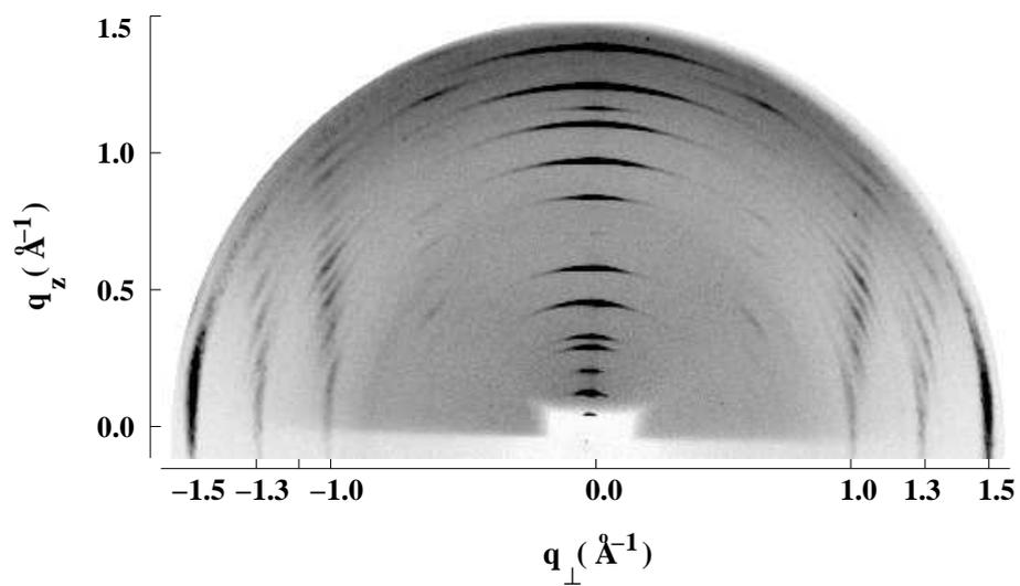
Figure 4.4: Diffraction pattern of a highly ordered phase of DLPE-cholesterol mixtures observed in a sample before heating to high temperatures ( $X_c = 10$  mol% ).
