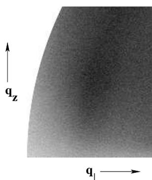
Figure 4.10: The wide angle reflection of DLPE-cholesterol mixture at  $X_c = 20$  mol% ( $T = 40^\circ\text{C}$ ,  $\text{RH} = 98\%$ ,  $d = 4.6$  Å).
