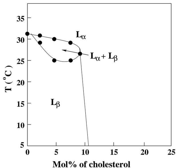
Figure 4.12: Partial phase diagram of DLPE–cholesterol mixtures at 98% RH, determined from the diffraction data collected on cooling.
