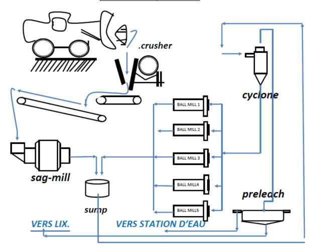
Figure 6 : Schematic of the fragmentation circuit
