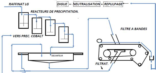
Figure13:Iron-Aluminum precipitation circuit
