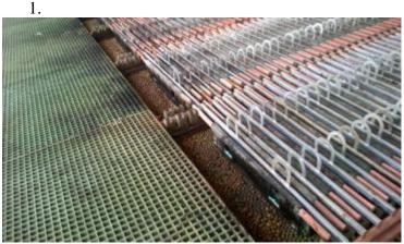
Figure 12: Pellets against gassing at electrolysis.
