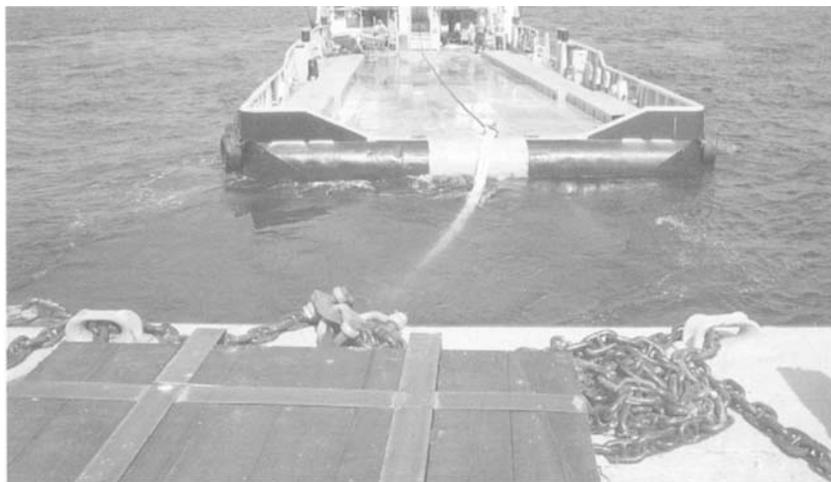
Figure 14.23 Typical arrangement of tow line and bridle
