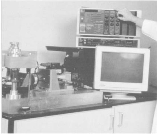
**Figure 16.67** Cyclic direct simple shear test
