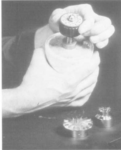
Figure 16.62 Torvane test
