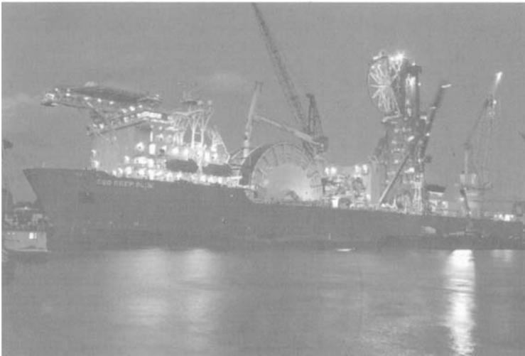
Figure 14.31 Deep Blue reel pipelay vessel
