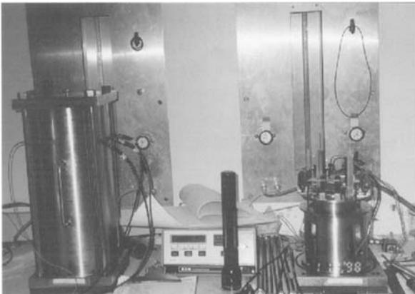
Figure 16.68 Resonant column test
