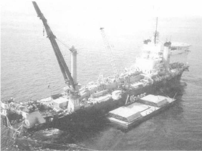
**Figure 11.17 Allseas Lorelay S-lay vessel – Courtesy C. Langner**
