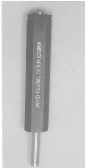
Figure 16.63 Pocket penetrometer
