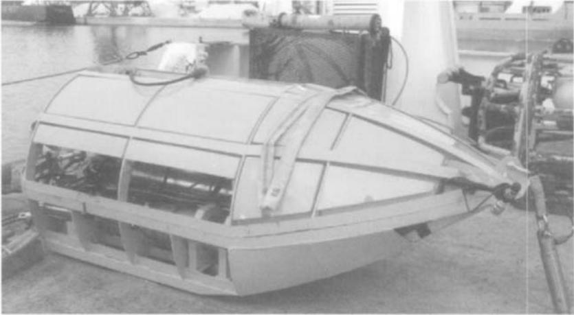
**Figure 16.15 GAMBAS<sup>®</sup> seismic refraction system – seabed tow sled**
