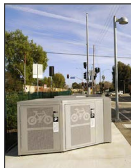
Figure 11: Bike Lockers Triangle-shaped bike lockers can vary in length but must have a mouth a minimum of 24" for clearance.
