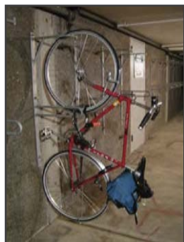
Figure 10: Vertical Bike Rack Dimensions are 2' wide and 6'4" tall. Racks should be distanced 24" from each other.
