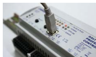
02 Commission the controller via USB connection to the PC
