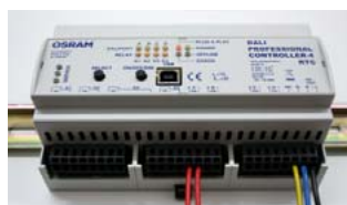
01 Mount the controller on the DIN rail and wire
