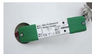
02 Pass the sensor coupler through the ceiling aperture
