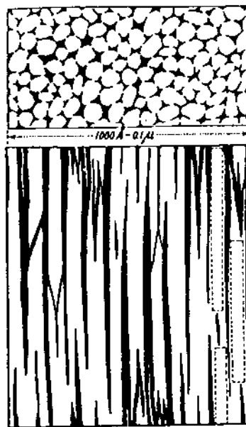
Figure 1.46 - Crystalline cellulosic structure. Frey-Wyssling . The upper part is a transverse section, the lower a longitudinal view. (The longitudinal view is greatly reduced in size, the crystalline regions being actually much more than ten times as long as wide). The dotted lines signify the crystalline regions through which the long-chain molecules pass and the black lines signify the voids.
