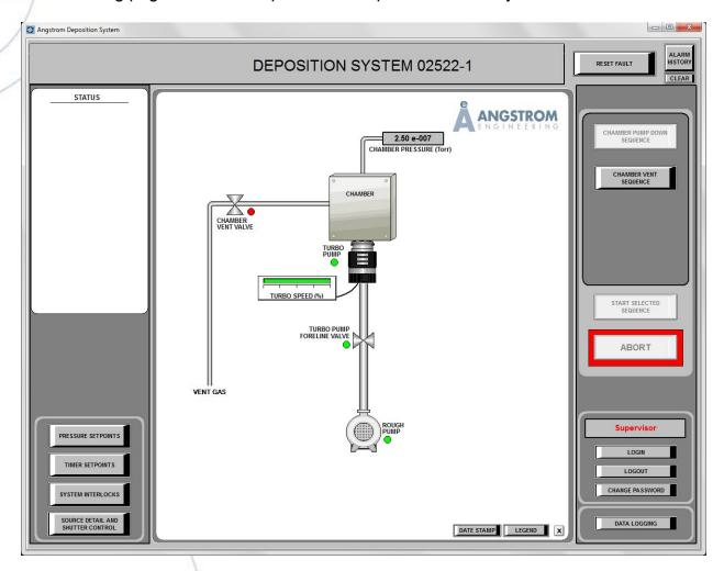
Shown above is the control software main page where all machine control is available except for deposition control. Deposition control is handled by the Inficon deposition software which opens as a separate program. See Chapter 4 – Depositing Materials for information on the Inficon deposition software.
