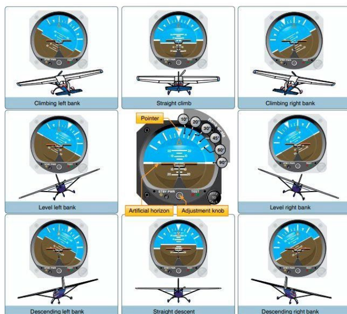
Figure 8-24. Attitude representation by the attitude indicator corresponds to the relation of the aircraft to the real horizon.
