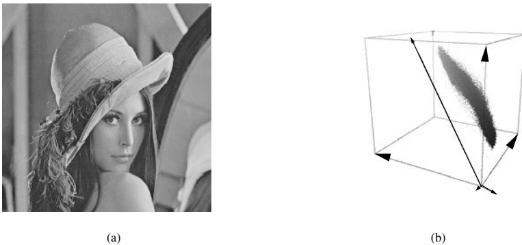
Figure 9.4 (See color insert following page 430) (a) Lenna test image and (b) its color set with the three eigenvectors ( v_1, v_2, v_3 ) of its covariance matrix. The length of each vector is proportional to its eigenvalue.
