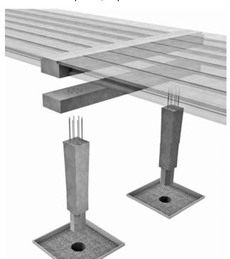
Figure 14.3.1.1-1 Precast Bent System, Exploded View
