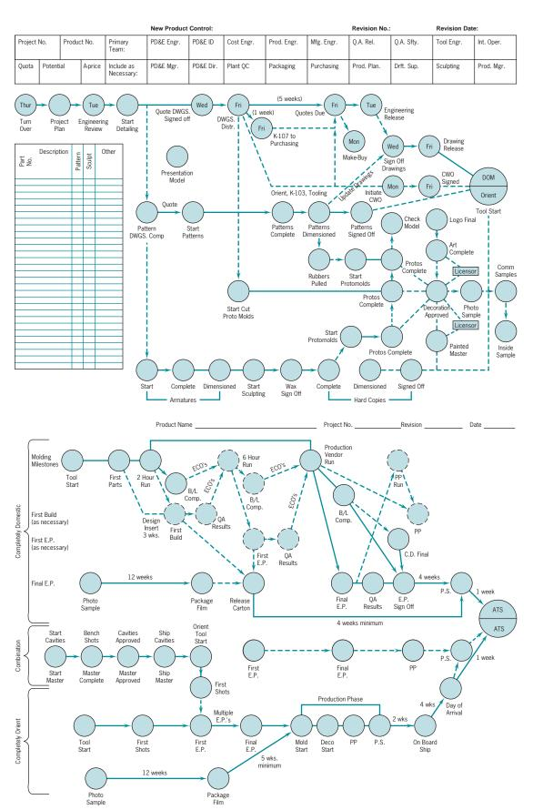
Figure 10-13 Sample project network with sign-off control.
