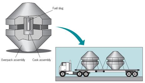
Fully assembled cask and transporting vehicle
