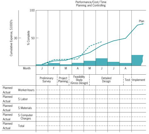
Figure 11-6 Integrated performance cost/time chart. Source: Murdick (1984).
