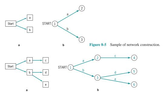
Figure 8-6 Sample of network construction.
