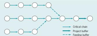
Figure 9-20 Project and feeder buffers.
