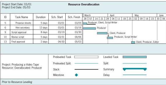
Figure 9-11 MSP load diagram showing resource conflict (producer used beyond capacity).
