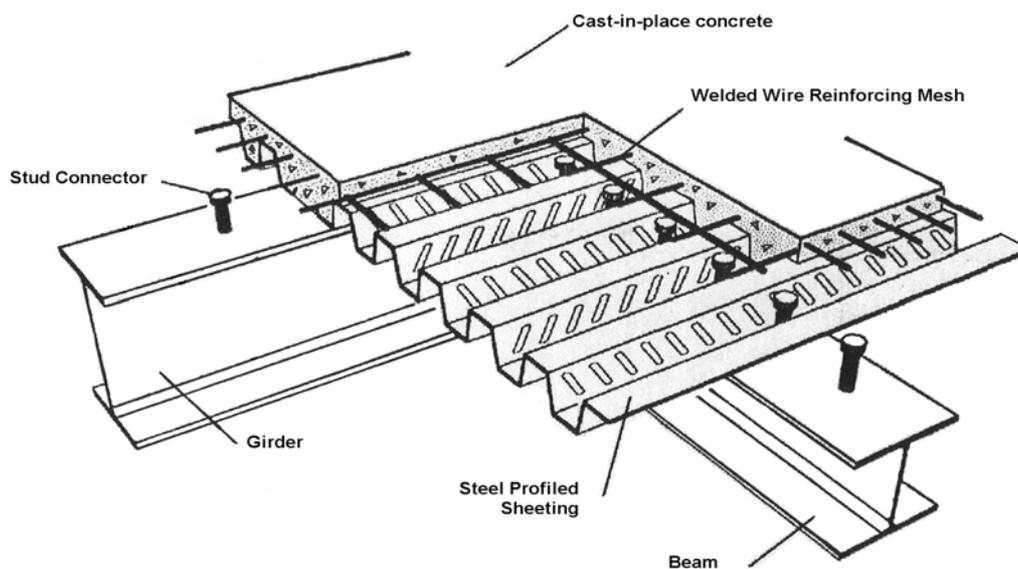
Figure 1. Details of composite profiled deck slab
