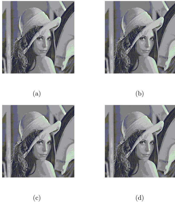
Figure 3.6: The quality of stego image when all parameters changes extremely.(a) p= 9976 bits, y= 2 , x= 2 , n=2 (b) p= 11584 bits, y= 3 , x= 3 , n=2 (c) p= 13320 bits, y= 4 , x= 4 , n=4 (d) p= 14352 bits, y= 5 , x= 5 , n=4
