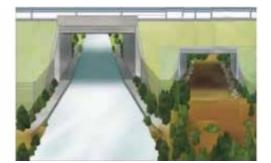
Fauna passage zones in box culvert, figure to the right shows an alternative dry passage, which does not alter the hydraulic properties of the structure.
