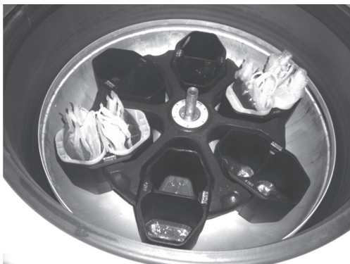
Figure 8.1: Cryofuge 6000i refrigerated centrifuge with blood bags bucket
