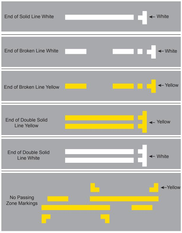
Figure 7-1 Spotting Symbols for Pavement Striping
