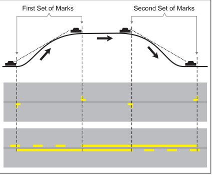
Figure 7-2 Establishing Marks for Identifying No-Passing Zone Locations
