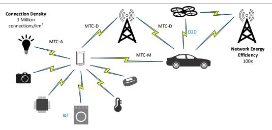
FIGURE 8. Massive Machine Type Communications (mMTC) provides efficient connectivity for the deployment of a massive number of geographically spread devices (e.g., sensors and smart devices). Three access types are planned for mMTC: direct network access (MTC-D), access via an aggregation node (MTC-A), and short-range D2D access (MTC-M).
