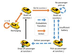
Fig. 2: An illustration of MDP for the computerized service strategy of an electric taxi.
