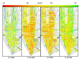
Fig. 4: Visualizations of driving speed networks.
