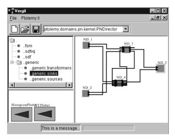
Figure 8: The derived PN network in the Ptolmey II framework.
