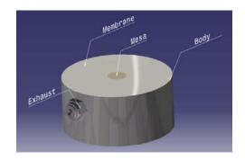
Figure 1: A general model of the sensing element.
