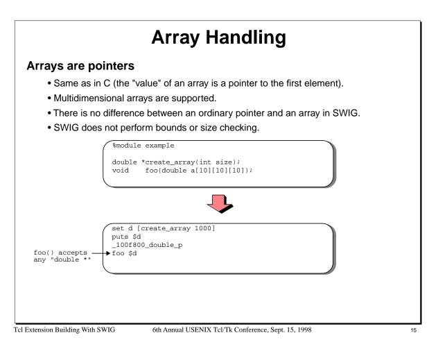
No checks are made to insure that arrays are of the proper size or even initialized properly (if not, you'll probably get a segmentation fault).
