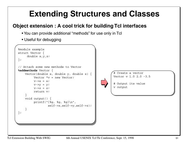
The object extension mechanism works with both C and C++. Furthermore, it does not rely upon any C++ magic nor does it affect the underlying objects in any way.
