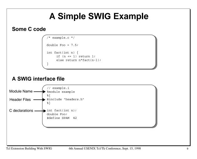
The % module directive specifies the name of the Tcl extension module.
