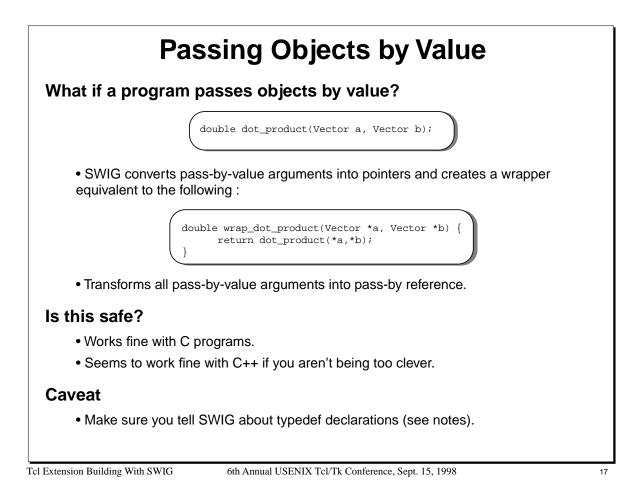
SWIG converts all undefined types into pointers. As a result, it is important to use typedef correctly. For example,
