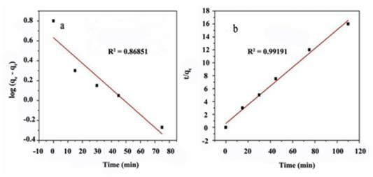
Figure 9. Adsorption kinetic for adsorption of Congored on NiO<sub>800</sub> (a) Pseudo-first order and (b)Pseudo-second order.
