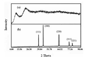
**Figure 4**. XRD patterns of (a) as-prepared Ni (II)/Chitosan hybrid (b) after calcination at 800 and 900°C.
