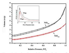
**Figure 5.**  $N_2$  adsorption and desorption isotherms of  $NiO_{800}$  and  $NiO_{900}$ . Inset is the corresponding pore size distribution of  $NiO_{800}$  and  $NiO_{900}$ .
