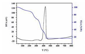
Figure 2. TGA and DTA curves of Ni-Chitosan hybrid.
