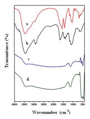
**Figure 1.** FTIR Spectra of (a) chitosan (b) as prepared Ni(II)/chitosan hybrid, (c) NiO nano spheres obtained after calcinations at 800 °C, for 6 h, (d) NiO nano spheres obtained after calcination at 900 °C, for 6 h.
