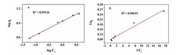
Figure 8. Adsorption isotherms for adsorption of Congored on NiO<sub>800</sub> (a) Freundlich and (b) Langmuir.
