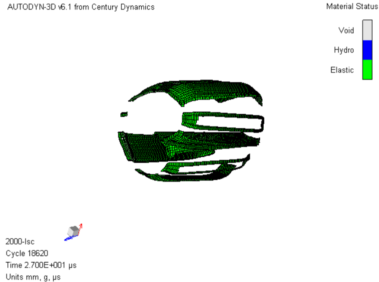
Figure 2-6. LSC 27 \mu sec after detonation (Lim, 2006). By this time the explosive has accelerated the entire length of the LSC liner. Notice how all the faces have been projected outwards (when compared to figure 2-5) and the blade has almost completely formed from the collapse of the LSC legs.
