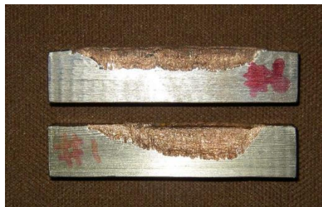
Figure 3-9. Linear initiation cut profile (top) single end initiation (bottom) (Lim, 2003). The cut profile of the linear initiation method shows that is performed worse than the single end initiation. There was no run-up observed and only a small amount of run-down on each end of the cut profile however the maximum cut depth was far less than the single point initiation method.
